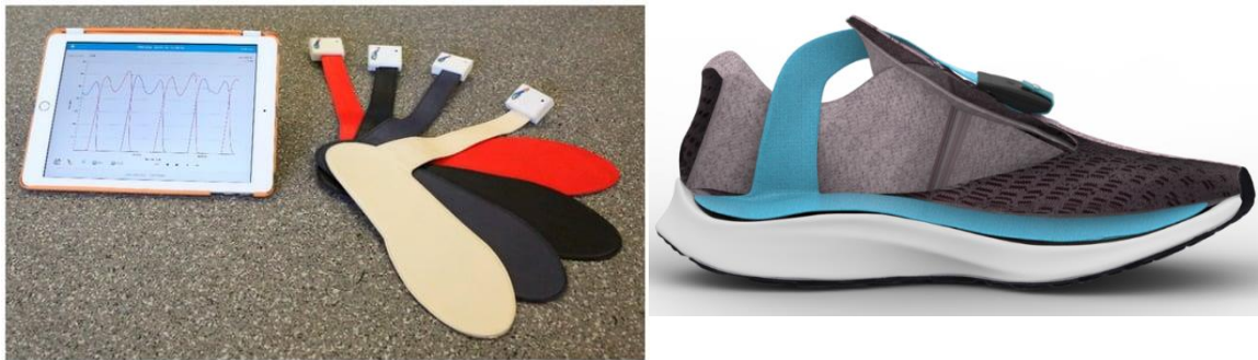
Figure 3: The loadsol ® and sample data (left) [16], loadsol inside shoe (right) [78]
