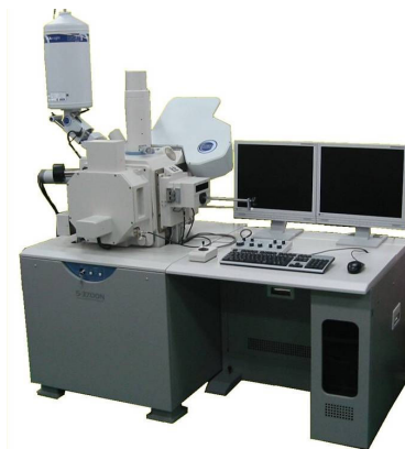
Figure 3.5 – Hitachi S-3700 Ultra Large Variable Pressure SEM used for imaging powder samples. [93]
