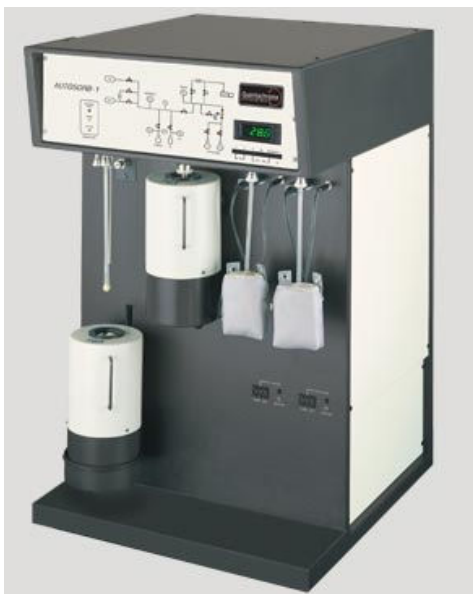
Figure 3.6 – Quantachrome Instruments Autosorb-1 Surface Area and Pore Size Analyzer used for determining surface area and pore volume. [94]
