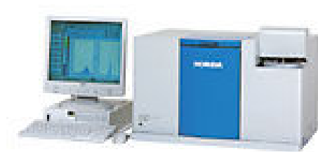
Figure 3.4 – Horiba Partica LA-950 Laser Diffraction Particle Size Analyzer used for determining the particle size distributions of SHS-produced \text{Al}_2\text{O}_3/\text{TiB}_2 powder. [92]
