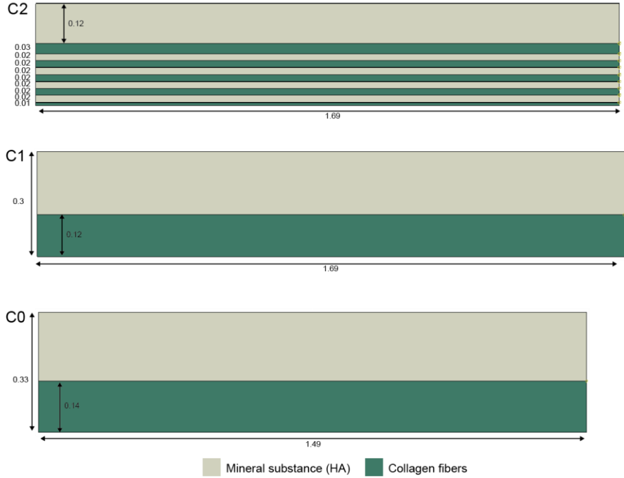
Fig. 6-10. The detailed dimension of the rectangular comparative FE simulation models. The upper model C2 is designed based on the cross-sectional structure of R2 model, the middle one C1 is designed based on the cross-sectional structure of R1 model, and the bottom C0 is designed based on the cross-sectional structure of F0 model.
