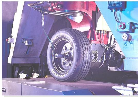
**Fig. 3-5 Flat-Trac test rig**
