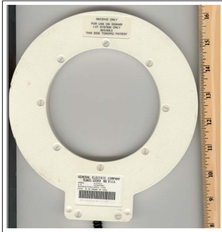
Figure 8. A medium to large size surface coil commonly used in orbital scans.
