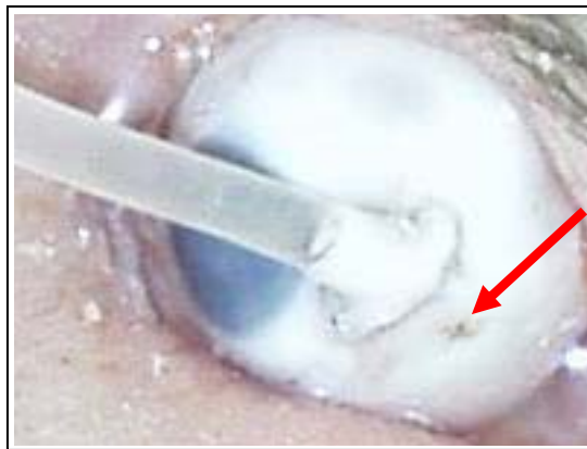
Figure 14. The arrow indicates the location where the sutures ripped through the sclera during a dynamic test utilizing a non-metallic catheter, which caused a leak.
