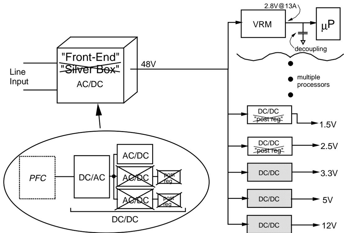
**Fig. 1.2 PC/workstation/server power supply architecture with a simplified silver box design.**
