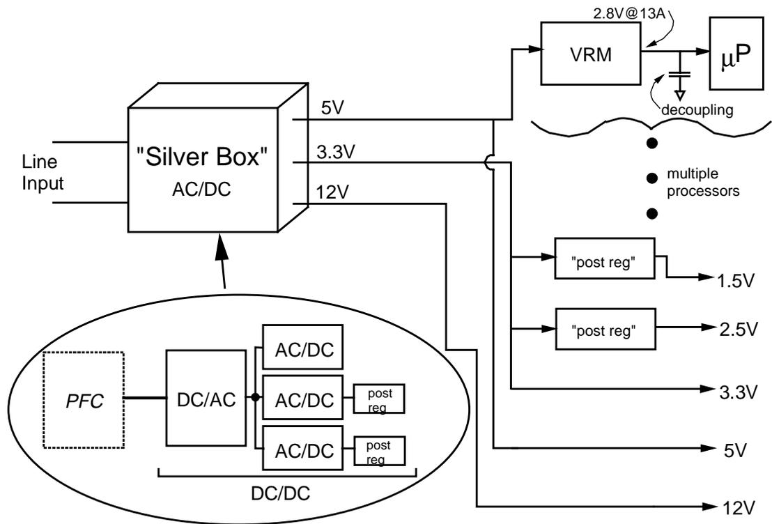
**Fig. 1.1 Typical present-day PC/workstation/server power supply architecture.**
