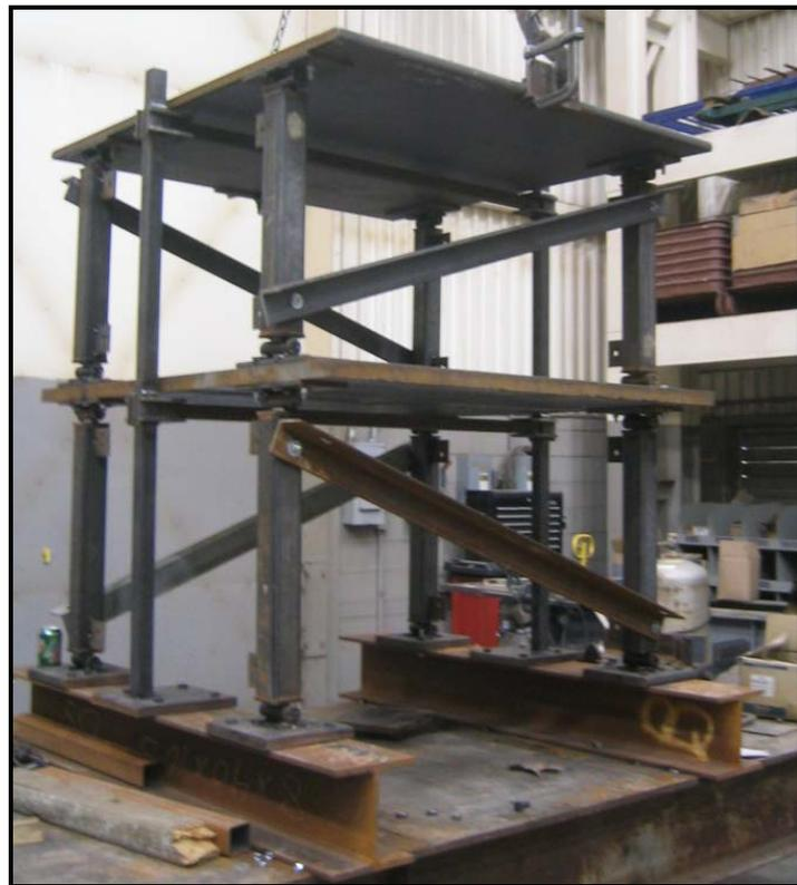
Figure 4. 4: Photograph of Mock-Up of Shaking Table Base Plate for Fit-Up at Irongate, Inc.
