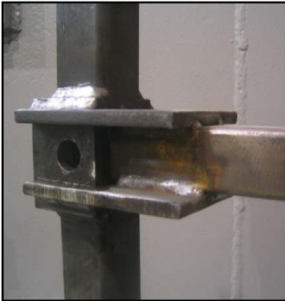
Figure 4. 6: Photograph of Connection at Beam-to-Column Joint
