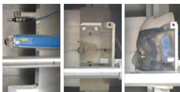
Figure 1: Boundary conditions. Left to right; isolated eye, synthetic orbit with eye, and 3D
