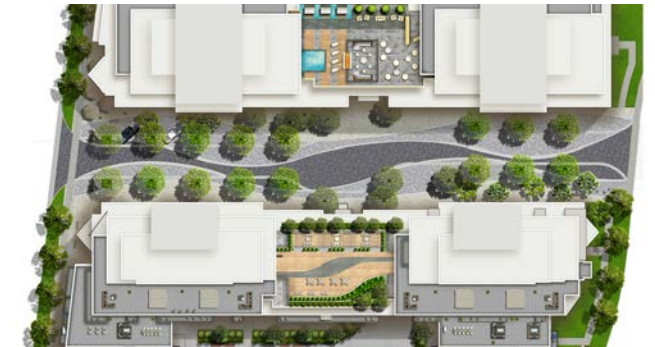
Oblique paving patterns can help create the meandering effect through the space
