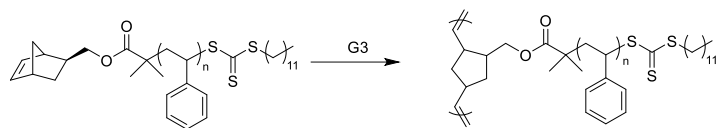
Scheme 5.2. ROMP of PS bottlebrush polymer targeting a backbone degree of polymerization equal to 500.
