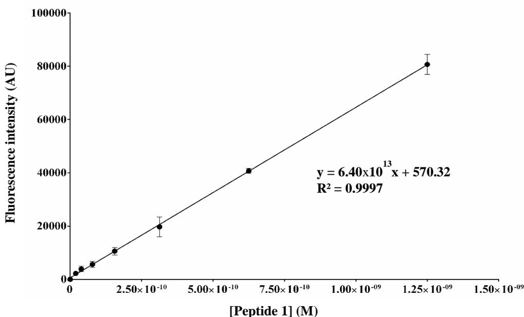
**Figure 2.7.** Calibration curve of peptide 1 in diluted DELFIA enhancement solution. Time-resolved fluorescence (TRF) was measured in a BioTek Cytation3 multimode reader with excitation at 340 nm and detection at 615 nm, 400  $\mu$ s delay time, 300  $\mu$ s collection time and gain of 200.
