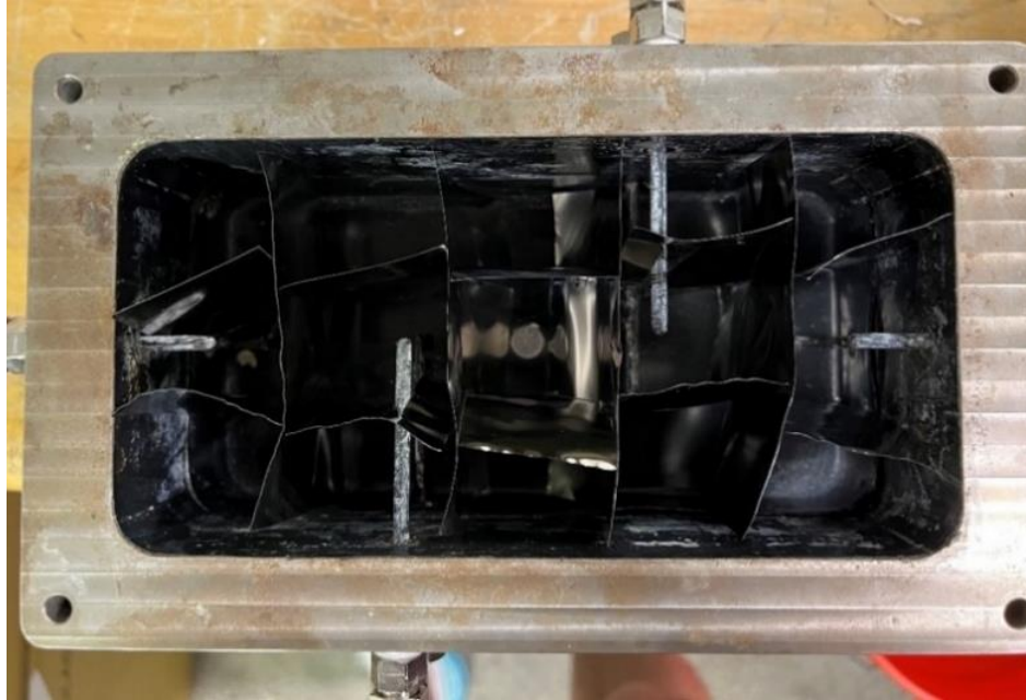
Figure 3.12: Steel foil fins inside hybrid box.
