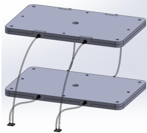
Figure 3.19: Rendering of the local coolant loop with piezoelectric pumps.
