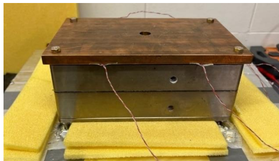
Figure 3.26: Hybrid control test setup without insulation
