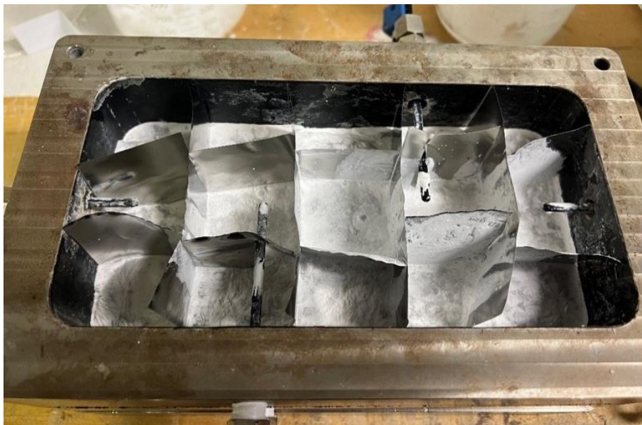
Figure 3.13: Solidified HS78 inside of hybrid box with the vertical steel foil fins.
