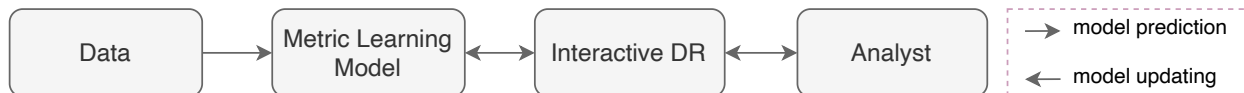
Figure 7.1: SI pipeline that follows the standard VA framework (adapted from [53, 143]). The interactive DR component serves as the visualization method responsible for capturing the analyst’s intent and updating the projection in response. The metric learning method [20] is the analytic model responsible for inferring the intents from interactive DR and providing the updated data relevance as feedback.
