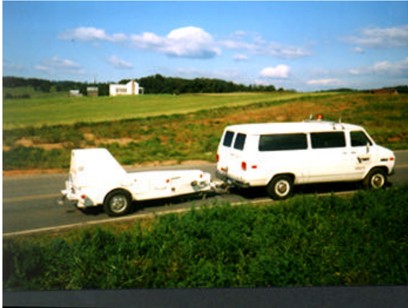
Figure 3.8 Falling weight deflectometer equipment
