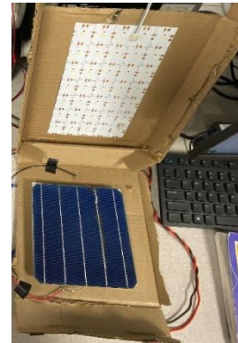
Figure 3-3 PV cell with LED sheet
