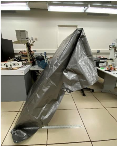
Figure 3-16 PV panel under dark condition
