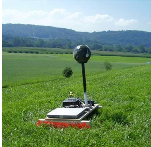
Figure 1.2: Acoustic node featuring a diffracting microphone array.
