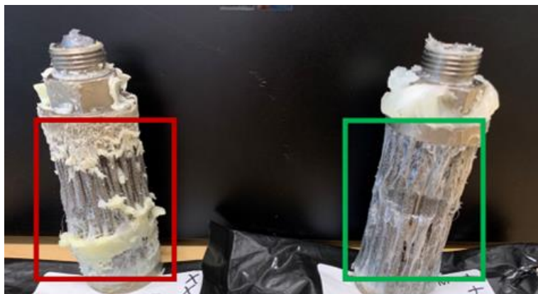
Figure 3.1: (Left) Solid white material building up on candle filters during extrusion and (Right) a candle filter without any particulate buildup, indicative of proper performance.
