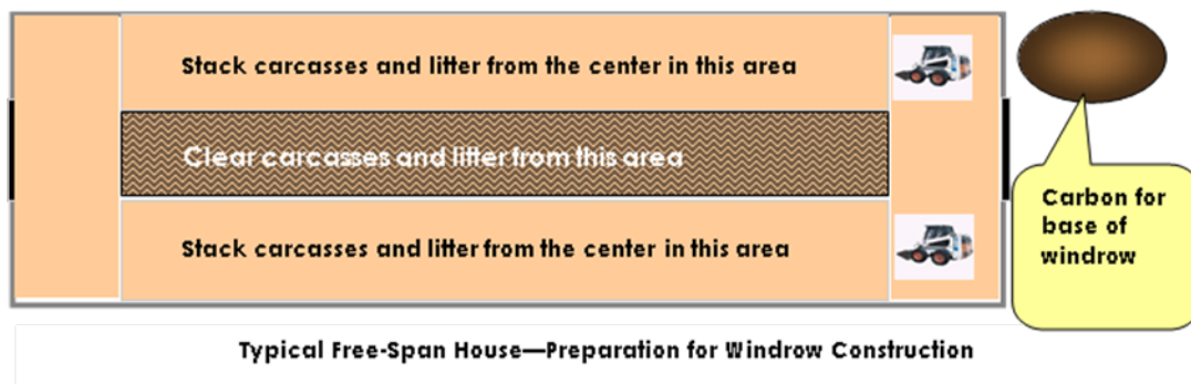
Figure 1. Preparation of work area for windrow construction in center of poultry house.
