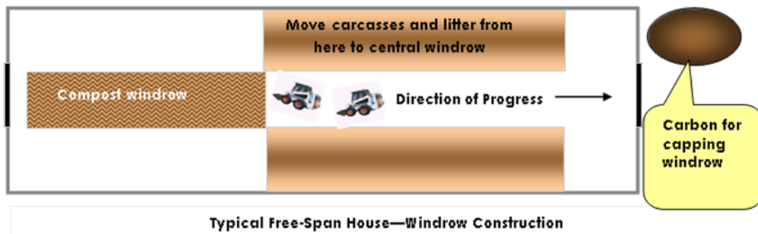
Figure 2. Beginning actual construction of windrow and direction of progress in a typical free-span house.
