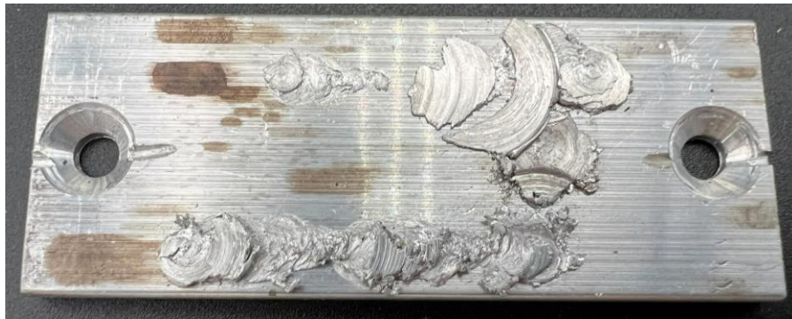
Figure 3. Several attempted aluminum depositions using aluminum 6061 feed rod onto 6061 substrate.
