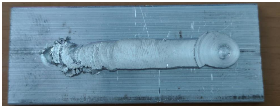
Figure 10. Aluminum 6061 feed rod on aluminum 6061 substrate deposition using the upgrade mill feeding mechanism with a preheated temperature of 420 °C.
