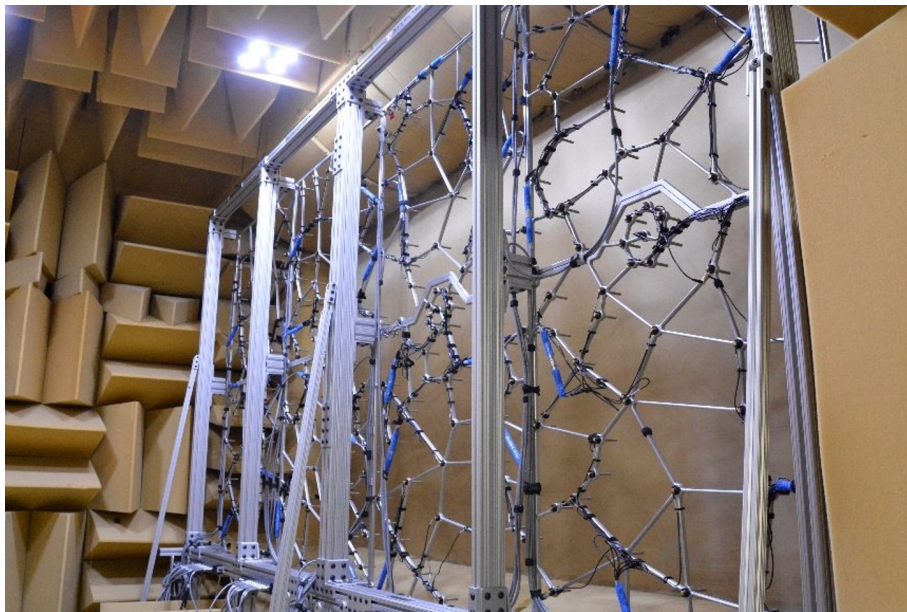
Figure 3.3: 251-channel microphone array configured in a single plane in the port side anechoic chamber of the Virginia Tech Stability Wind Tunnel
