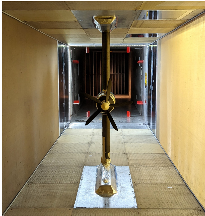
Figure 5.1: Scaled propeller in the axial flight configuration ( \Psi = 0^\circ )
