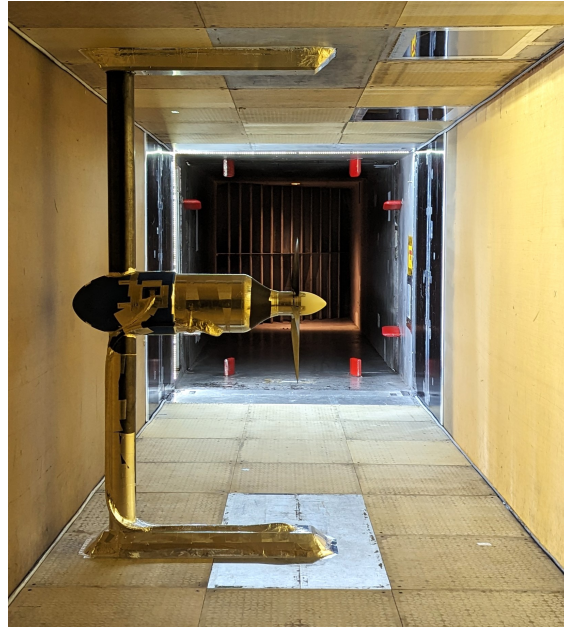
Figure 5.4: Scaled propeller in the edgewise flight configuration ( \Psi = 90^\circ )
