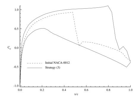
Figure 6.7: Results from the reformulated design problem (M  $_{\star}$  = 0.8, a  $_{\star}$  = 0 ).
