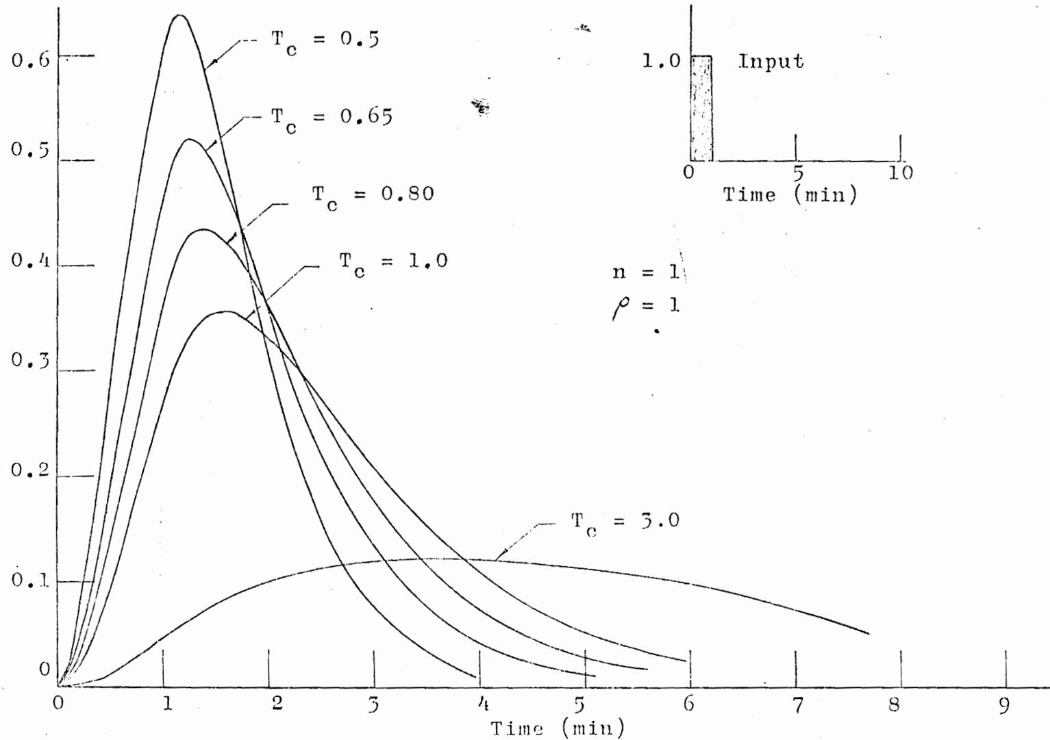
Figure 5-19. Effect of Varying Time Constant  $T_c$  on Outflow for A Second Order System ( $n = 1, \rho = 1$ ).
