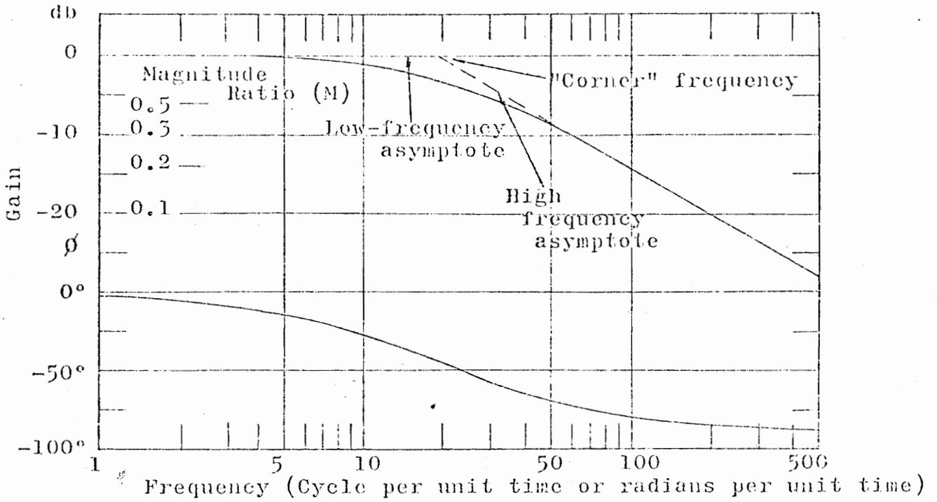
Figure 4-2. Typical Bode Diagram for First Order System.
