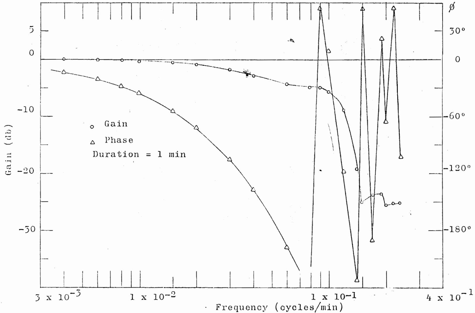
Figure 5-16. Bode-Diagram for S = 2%, R = 1.26 in/hr, Basin Type III.
