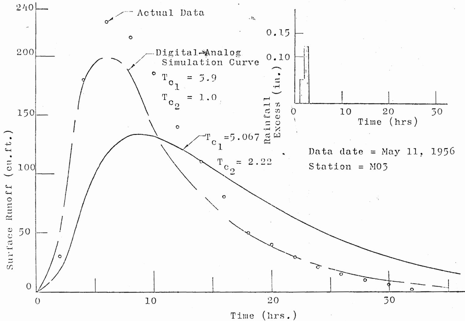
Figure 5-28. Comparison of Actual Data with Digital-Analog Simulation Curve.
