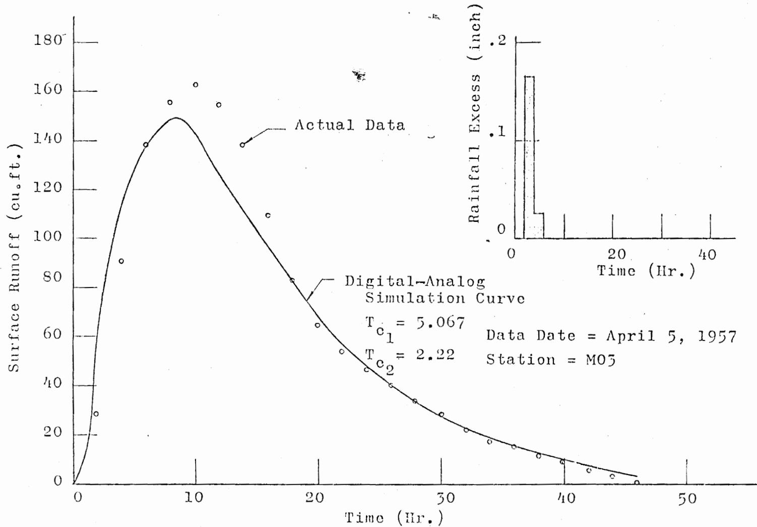
Figure 5-27. Comparison of Actual Data with Digital-Analog Simulation Curve.
