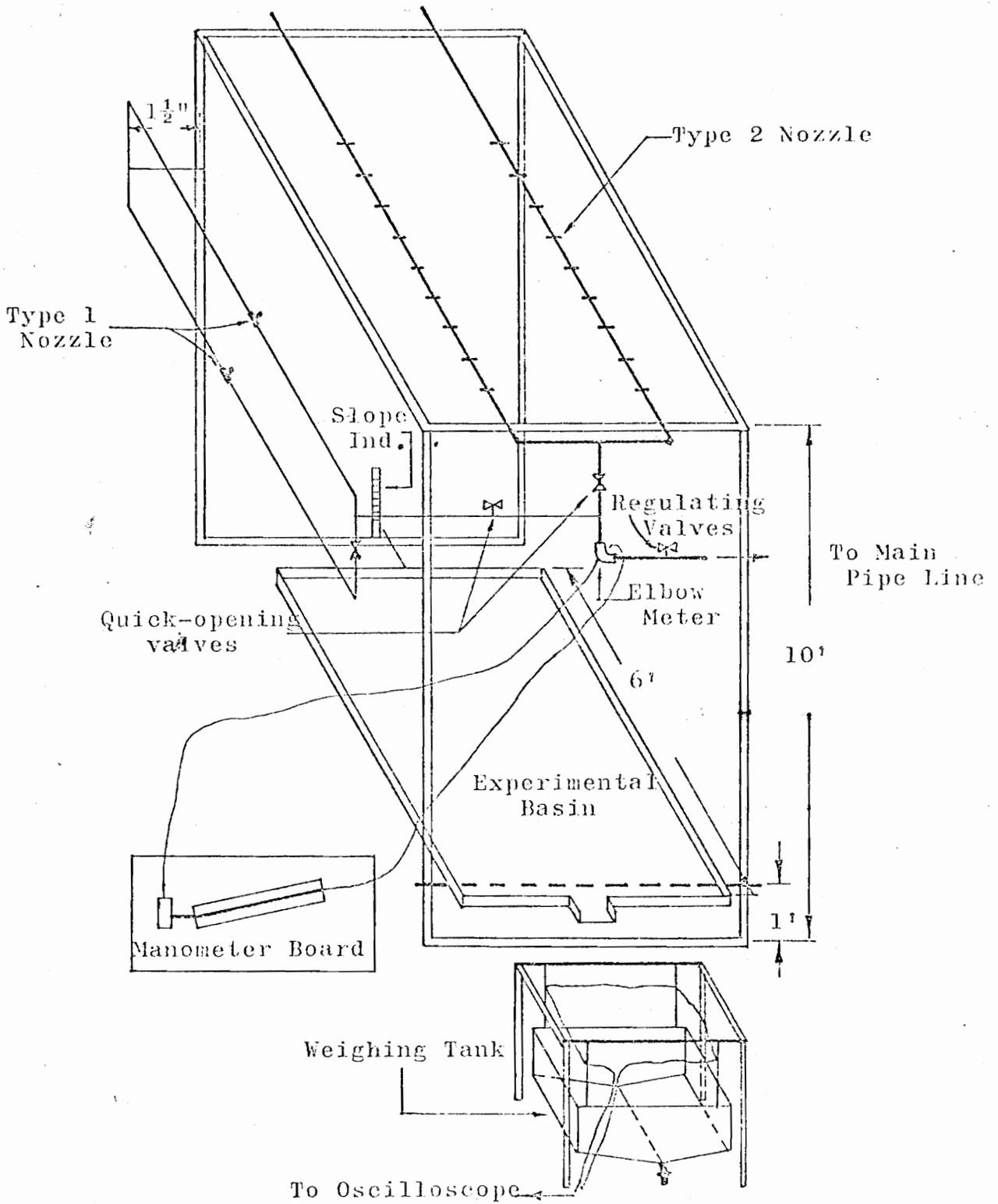
Figure 3-2. Sketch of Experimental Basin and Measurement Devices.
