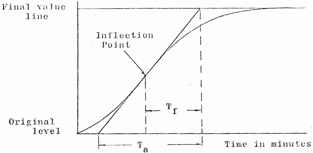
Figure 5-17. Typical Process Reaction Curve (Dead Time Neglected).
