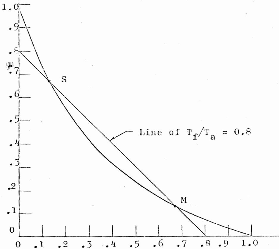
Figure 5-18. Graph for Finding Equivalent Time Constant from Process Reaction Curve. (After Tucker and Wills(45)).
