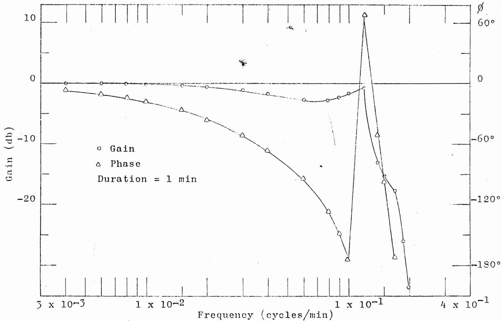
Figure 5-13. Bode-Diagram for  $S = 8\%$ ,  $R = 1.26$  in/hr, Basin Type III.
