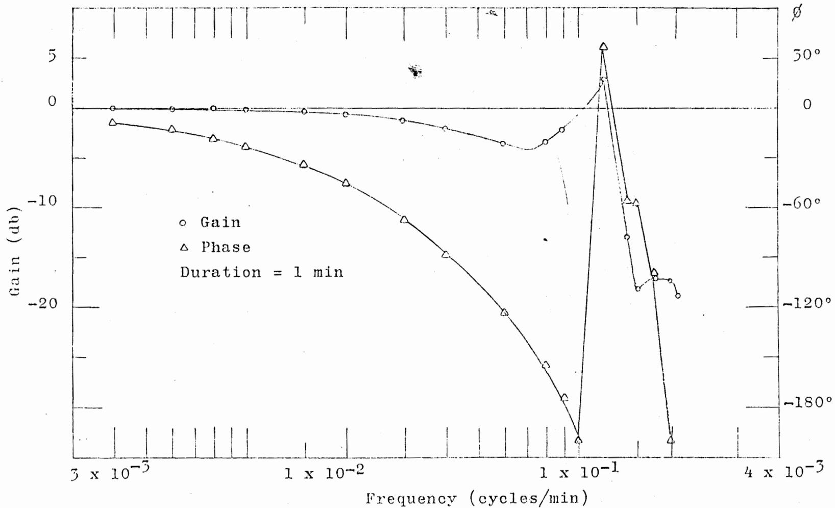
Figure 5-15. Bode-Diagram for S = 4%, R = 1.26 in/hr, Basin Type III.
