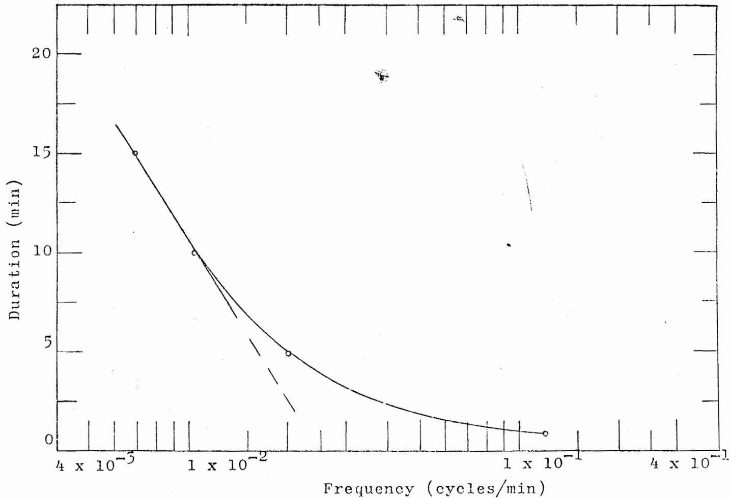
Figure 5-10. Relationship Between Maximum Frequency of Gain Curve and Input Duration.
