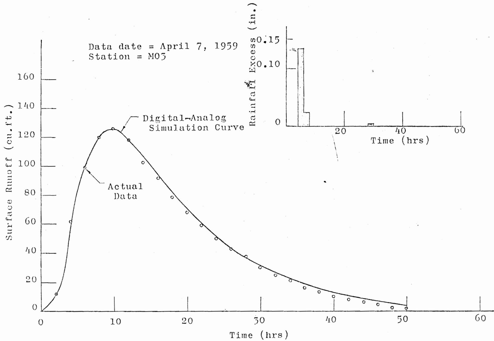
Figure 5-26. Comparison of the Actual Data with Digital-Analog Simulation Curve.
