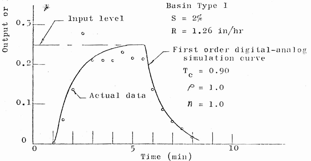
Figure 5-24. Comparison of Digital-Analog Simulation and Actual Data by First Order, Linear System for Basin Type I,  $S = 2\%$ .
