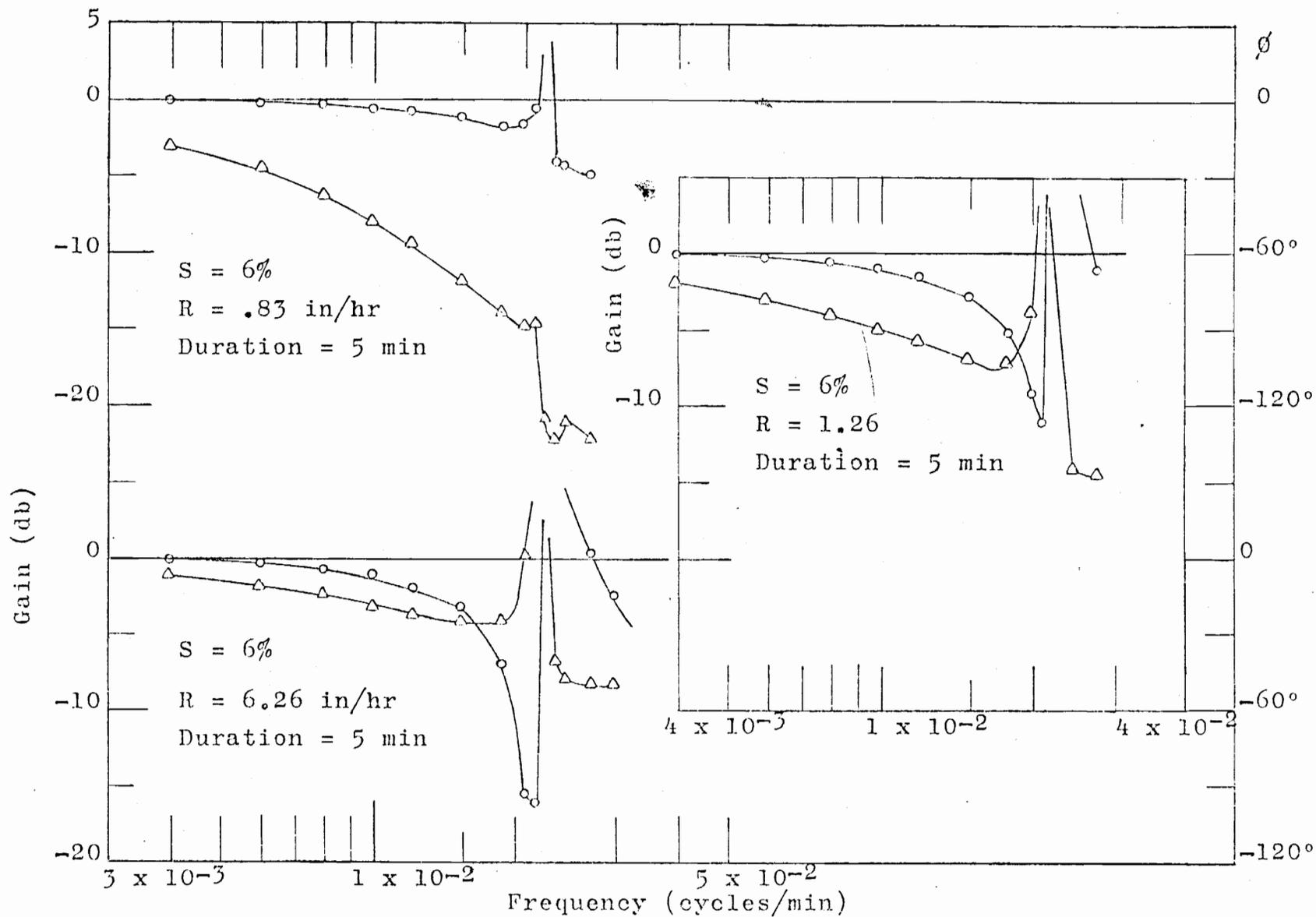
Figure 5-12. Bode-Diagram for Input Intensity Varying at  $S = 6\%$ , Basin Type III.
