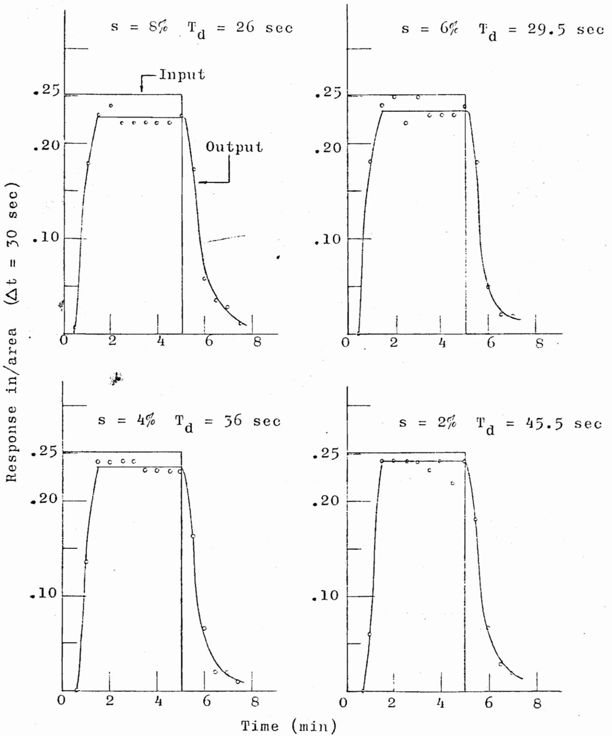
Figure 5-5. Response for Basin Type III for  $R = 1.26$  in/hr for Various Slopes.
