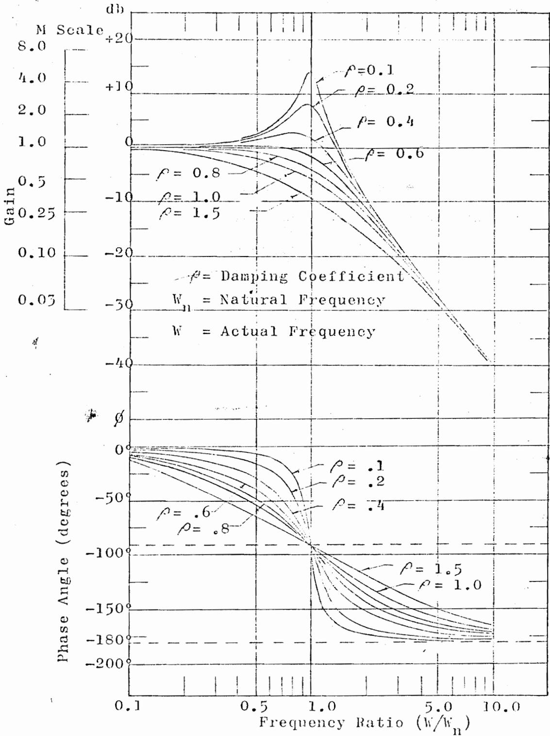
Figure 4-4. Frequency Response of Second-Order Systems Showing Damping Coefficients for Various Gain Curves and Phase Angle Curves.
