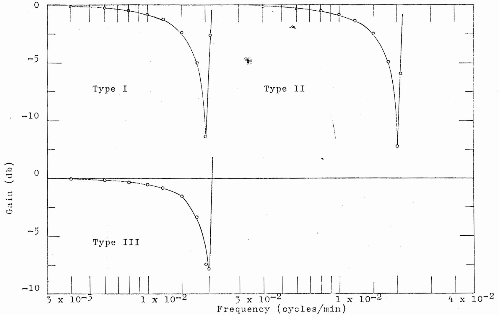
Figure 5-11. Gain Curves for Different Basin Types at  $S = 8\%$ ,  $R = 6.26$  in/hr.
