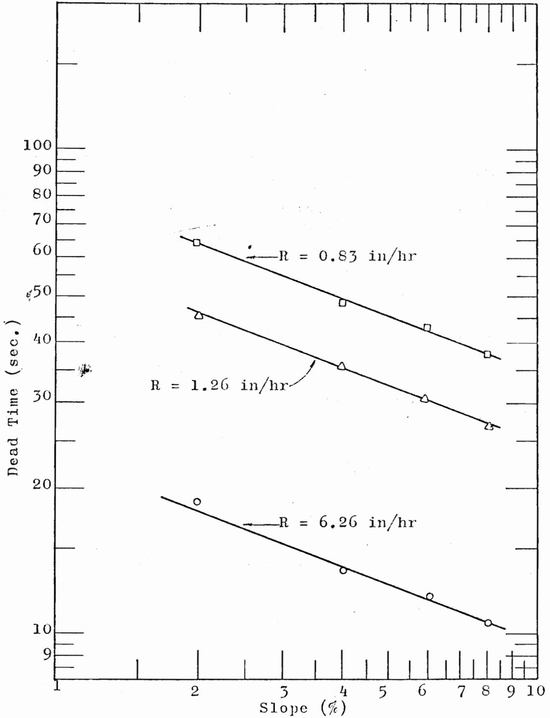
Figure 5-4. Relationship Between Dead Time and Basin Slope for Basin Type III.
