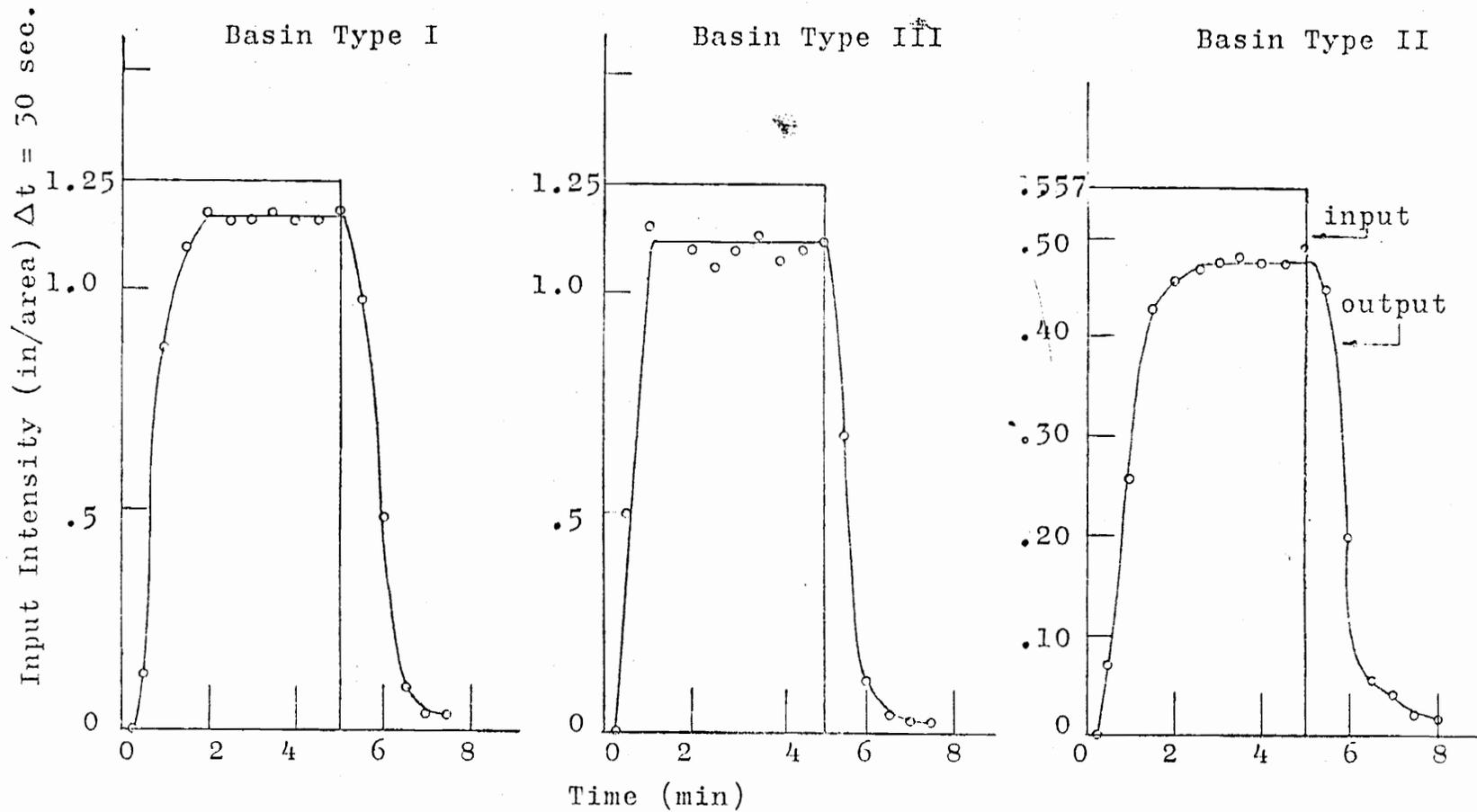
Figure 5-8. Response for Basin Type Varying,  $R = 6.26$  in/hr,  $S = 4\%$ .
