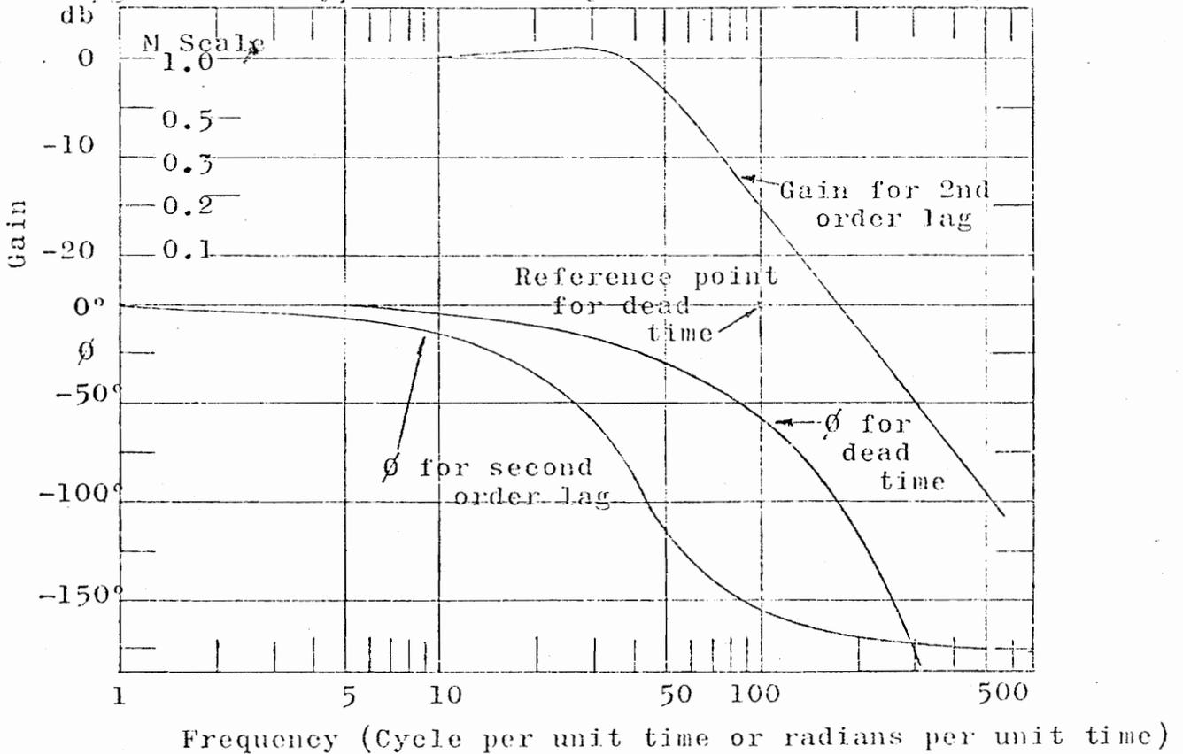
Figure 4-5. Typical Bode Diagram for Second Order System.
