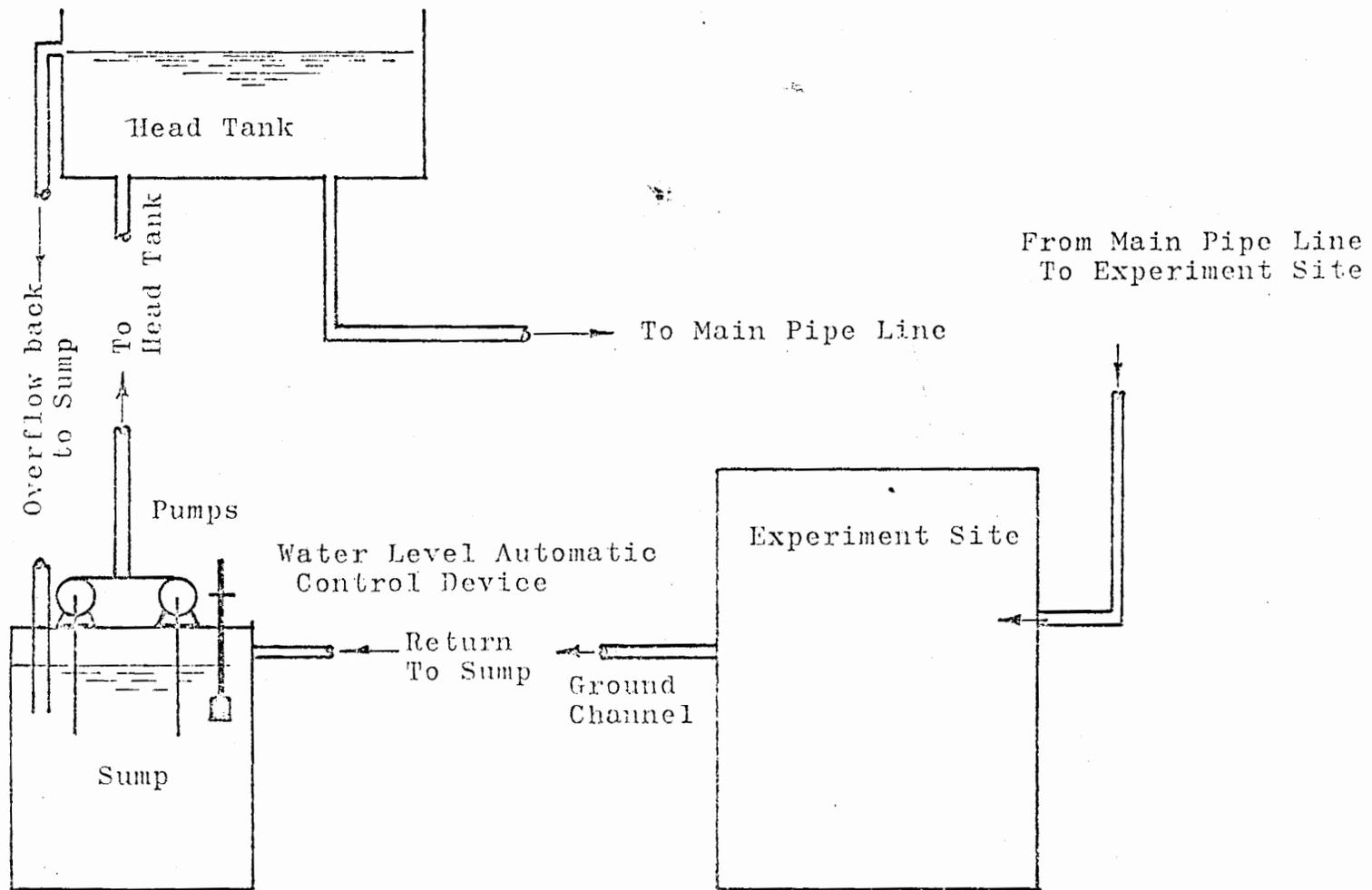
Figure 3-1. Sketch of Water Supply System.
