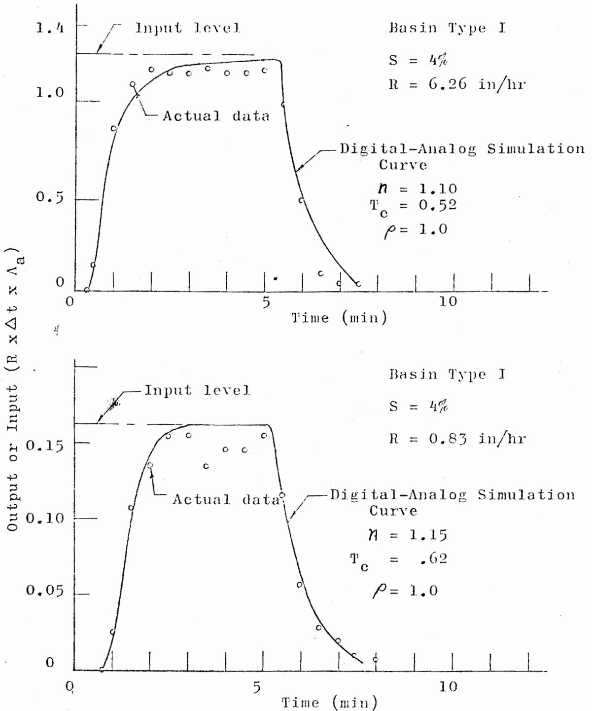
Figure 5-25. Comparison of Digital-Analog Simulation Curve and Actual Data for Input Intensity Varying.
