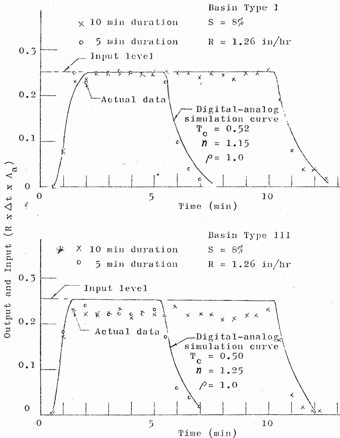
Figure 5-22. Comparison of Digital-Analog Simulation Curve and Actual Data for Duration Varying.
