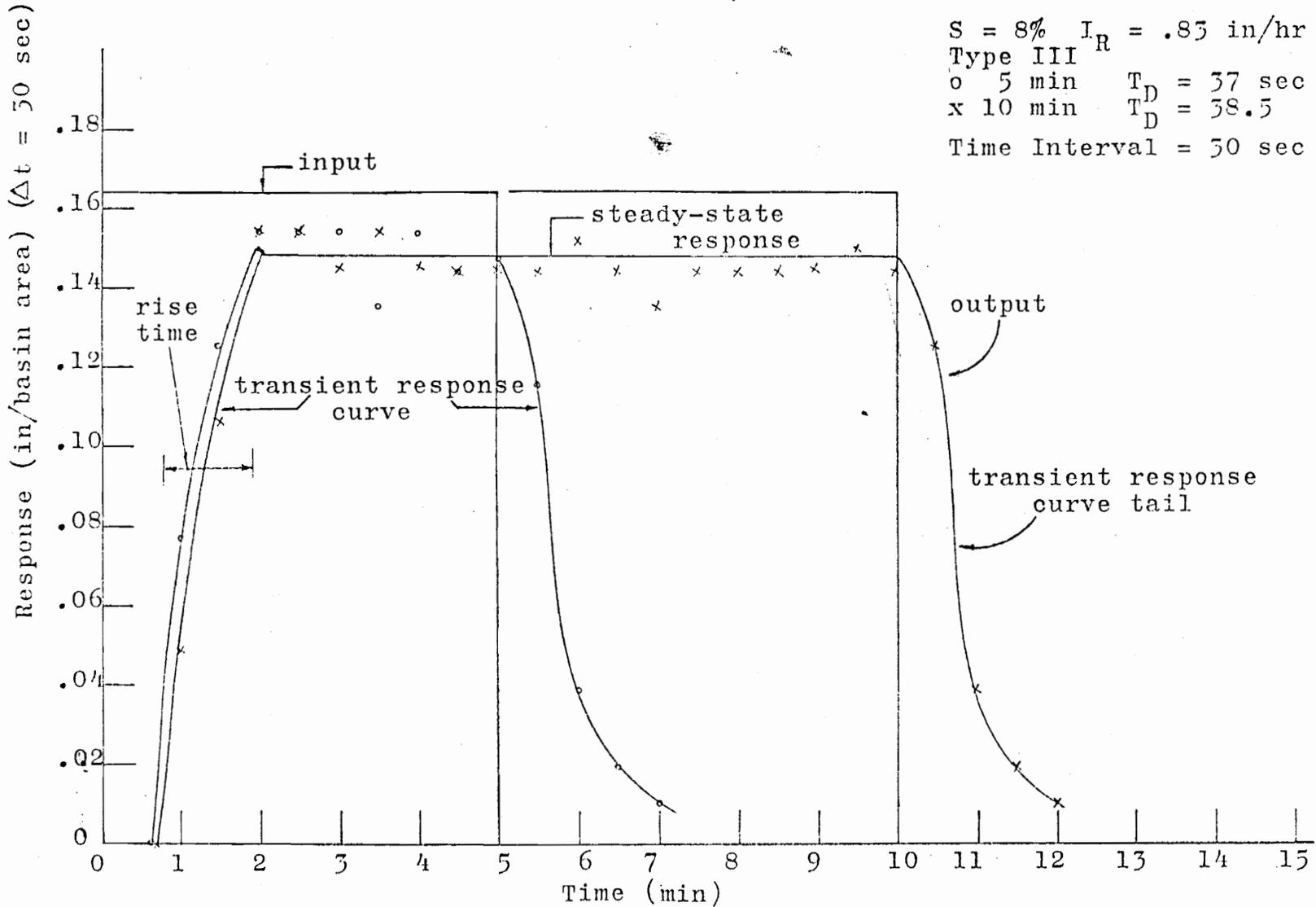
Figure 5-6. Response for Different Durations (Basin Type III,  $S = 8\%$ ,  $R = .85$ )
