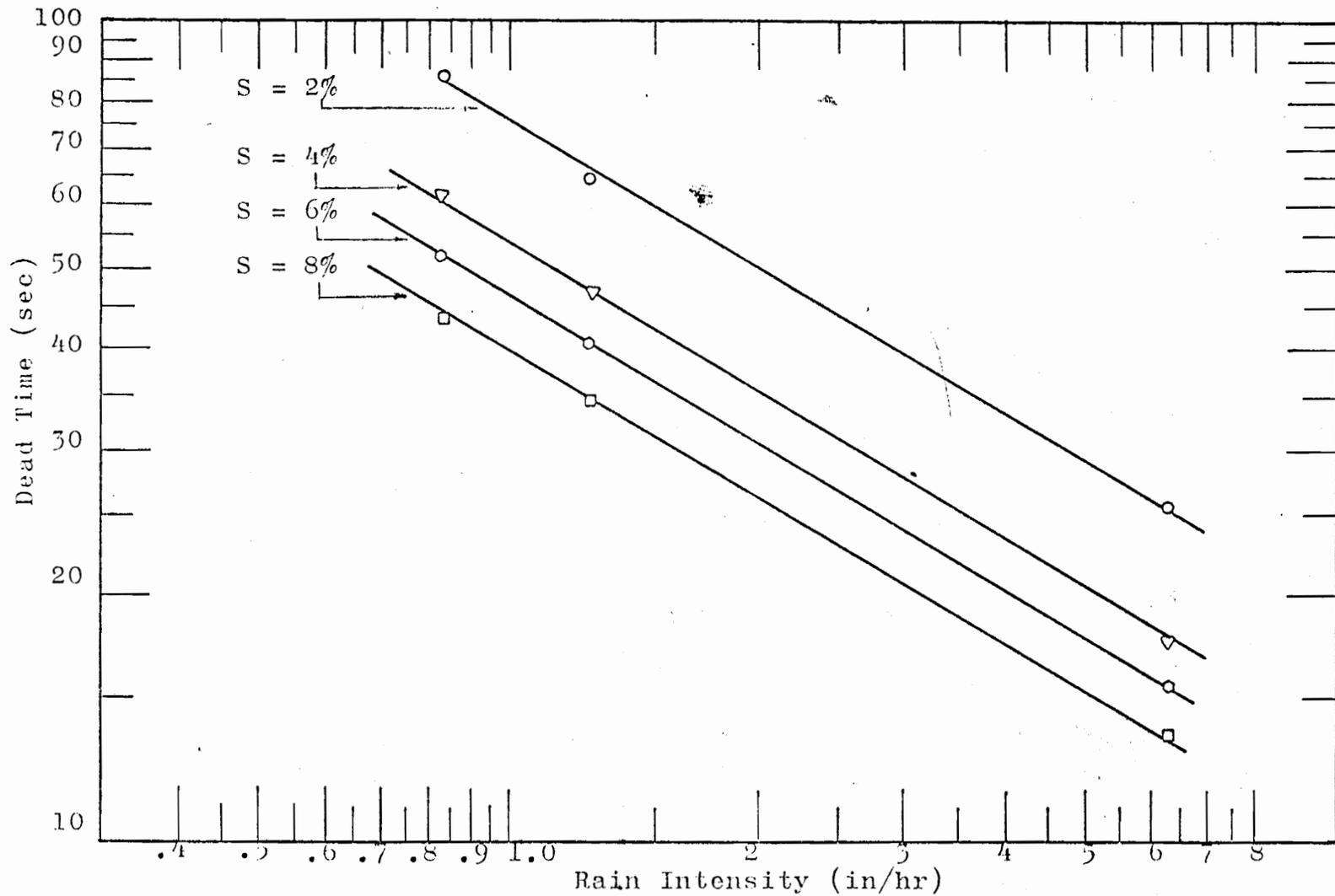
Figure 5-1. Relationship Between Dead Time and Rain Intensity for Basin Type I.
