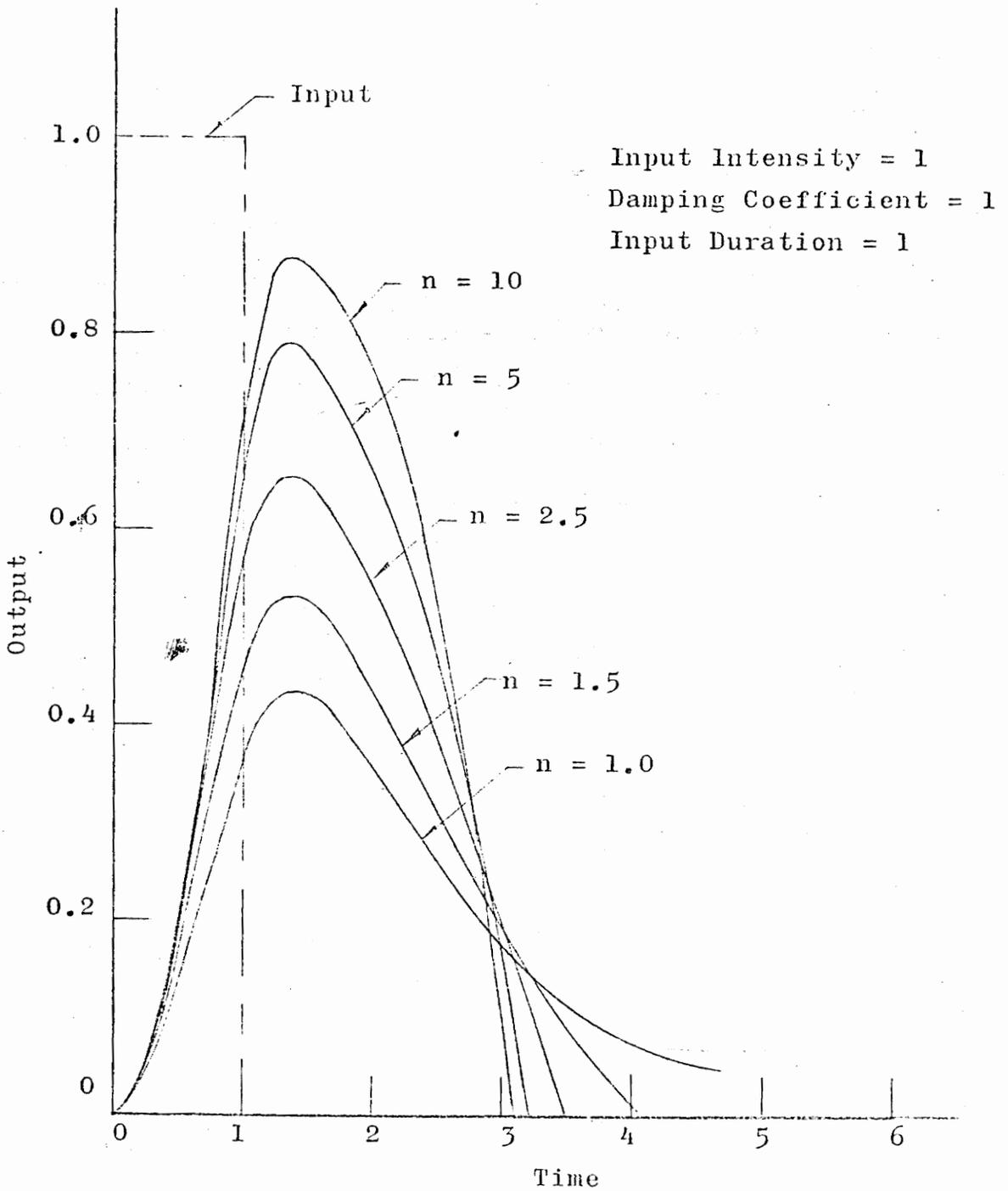
Figure 5-20. Effect of Varying  $n$  on Outflow for A Second Order Nonlinear System.
