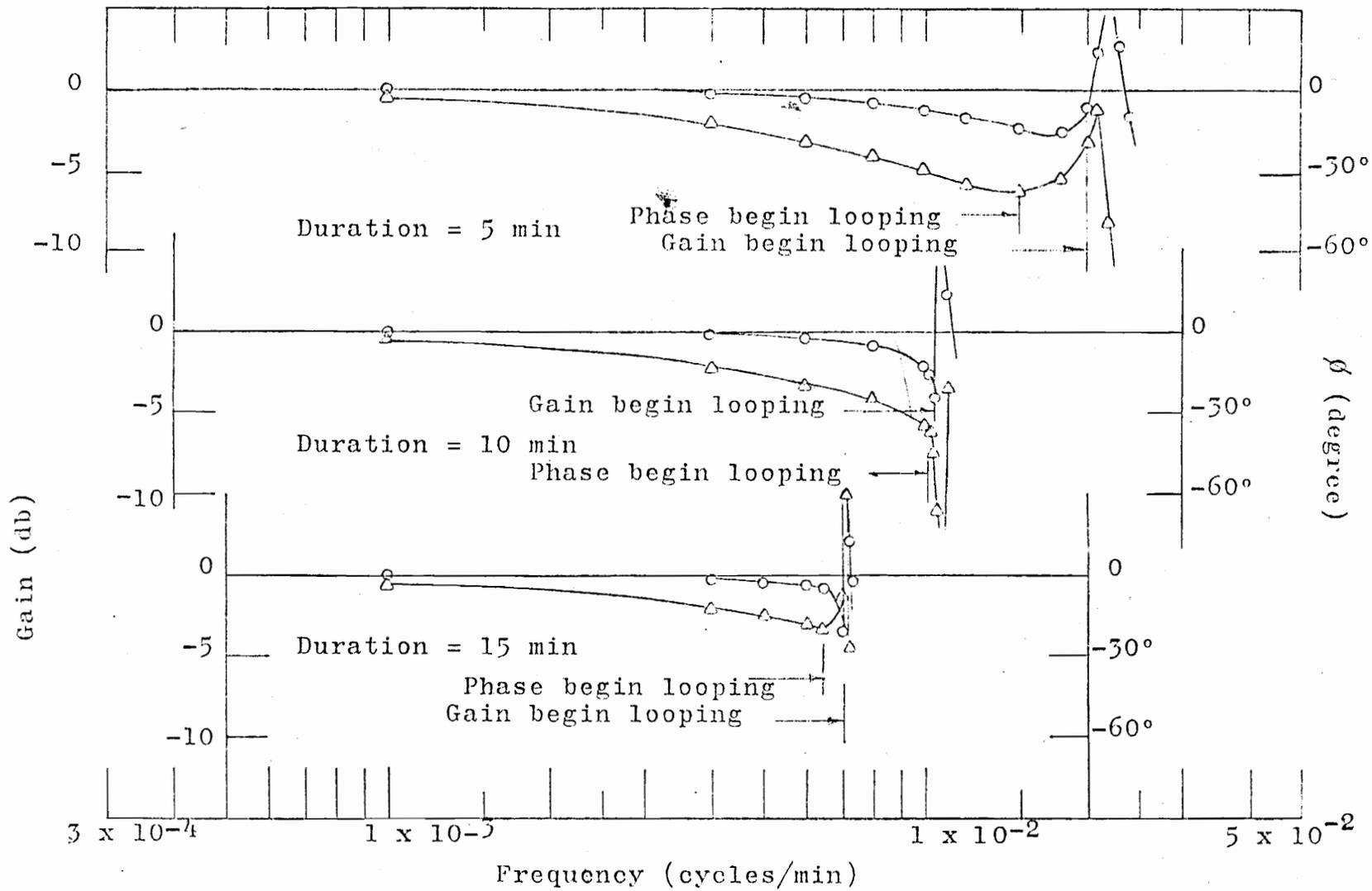
Figure 5-9. Bode Diagram for Varying Durations, Basin Type I, R = 1.26 in/hr
