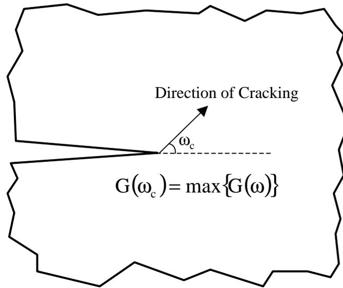
**Fig. 3.** The direction of crack propagation can be determined by maximizing the strain energy release rate as a function of the crack kinking angle.
