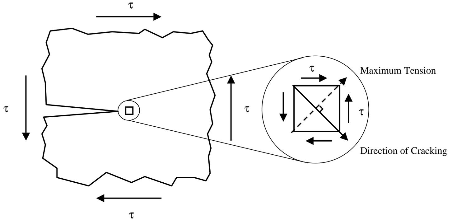
**Fig. 2.** A crack under pure shear loading. The direction of crack propagation is perpendicular to the direction of maximum tension.
