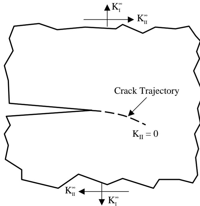
**Fig. 4.** For a crack under mixed mode loading, the crack will propagate along a trajectory such that mode I fracture is maintained at the crack tip.
