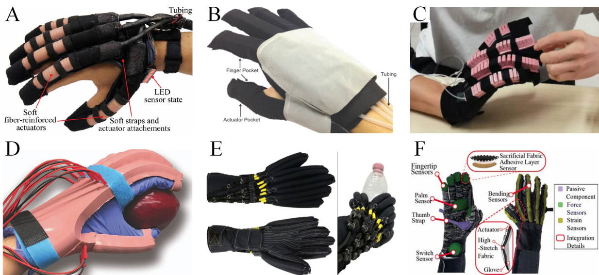
Figure 1.2: Soft robotic exoskeleton glove system in the last decade. The compliant inflatable elastic segments actuated by the pneumatic actuators cover the whole hand.
