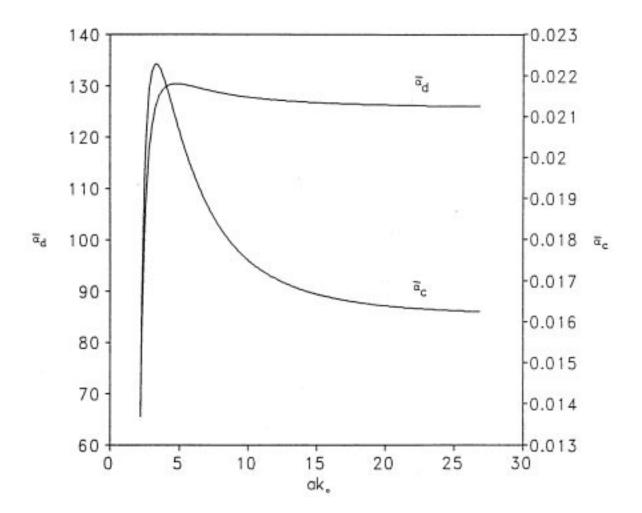
Figure 5.5 Variations of normalized attenuation coefficients of conductor,  $\alpha_c$ , and dielectric,  $\alpha_d$ , versus normalized frequency,  $\alpha k_o$ , for the  $TE_{01}$  mode in a wedge-shape dielectric waveguide with  $\phi_o = \pi/n$ ; n an integer, and  $\epsilon_{r1} = 2.25$ , and  $\epsilon_{r2} = 1$ .
