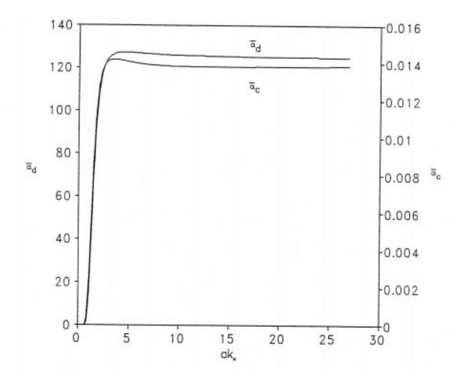
Figure 5.3 Variations of normalized attenuation coefficients of conductor,  $\alpha_c$ , and dielectric,  $\alpha_d$ , versus normalized frequency,  $\alpha k_o$ , for the  $HE_{11}$  mode in a wedge-shape dielectric waveguide with  $\phi_o = \pi$ , and  $\epsilon_{r1} = 2.25$ , and  $\epsilon_{r2} = 1$ .
