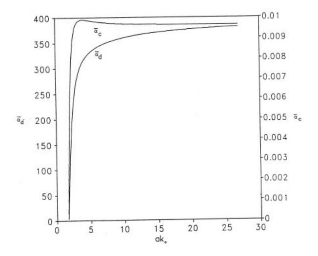
Figure 5.4 Variations of normalized attenuation coefficients of conductor,  $\alpha_c$ , and dielectric,  $\alpha_d$ , versus normalized frequency,  $\alpha k_o$ , for the  $HE_{3/2,1}$  mode in a wedge-shape dielectric waveguide with  $\phi_o = 2\pi/3$ , and  $\epsilon_{r1} = 2.25$ , and  $\epsilon_{r2} = 1$ .
