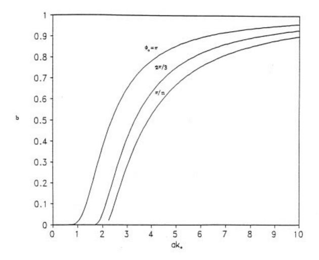
Figure 5.2 Normalized propagation constant, b, versus normalized frequency,  $\alpha k_o$ , for the fundamental modes of wedge-shape dielectric waveguide with  $\phi_o = \pi$ ,  $2\pi/3$ , and  $\pi/n$ ;  $n \geq 2$ , and with  $\epsilon_{r1} = 2.25$ , and  $\epsilon_{r2} = 1$ . The fundamental modes for these values of  $\phi_o$  are  $HE_{11}$ ,  $HE_{3/2,1}$ , and  $TE_{01}$ , respectively.
