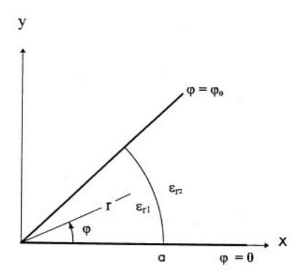
Figure 5.1 Geometry and coordinates for a wedge-shape dielectric waveguide bounded by conducting planes at  $\phi=0$  and  $\phi=\phi_o.$
