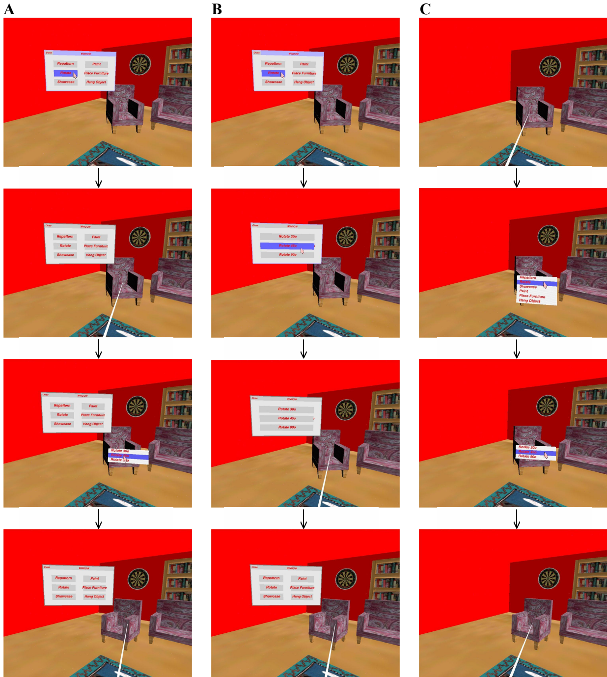
Figure 3.2 Implementations of a rotate command with a 45° parameter using A) the Action-Object-Parameter task sequence, B) the Action-Parameter-Object task sequence, and C) the Object-Action-Parameter task sequence.
