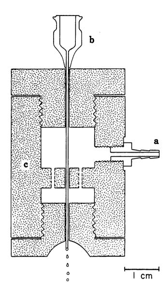
Figure 2. Two-dimensional drawing of self-centering encapsulating jet; (a) Air inlet nozzle, (b) 22 gauge stainless steel needle, (c) Nylon polymer casing.
