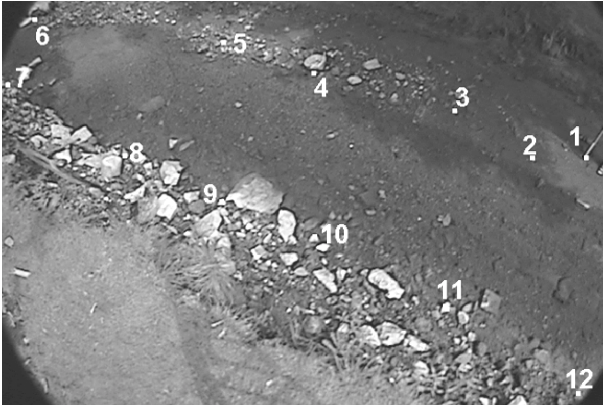
Figure 20. Twelve temporary GRP shown for the Stroubles Creek field site (picture enhanced for clarity). The points were necessary to register and transform the image to remove spatial distortion.
