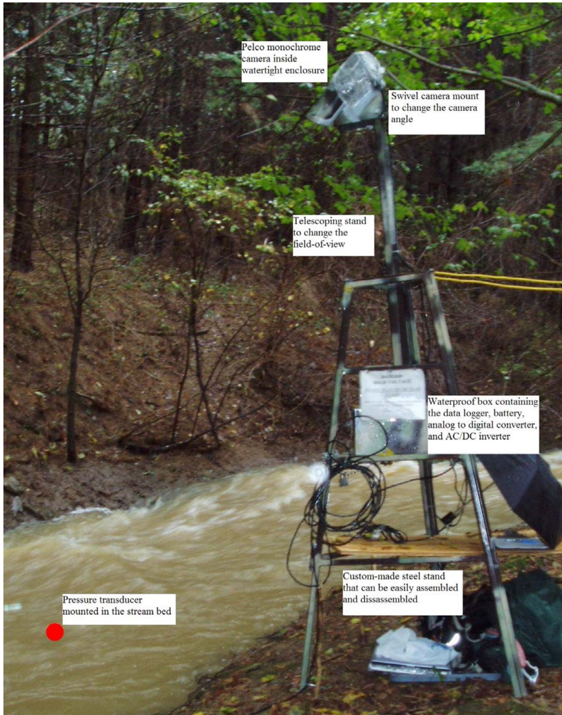
Figure 24. A photo of the LSPIV prototype in use at Crab Creek. The prototype was transportable and could be used for a variety of site conditions.
