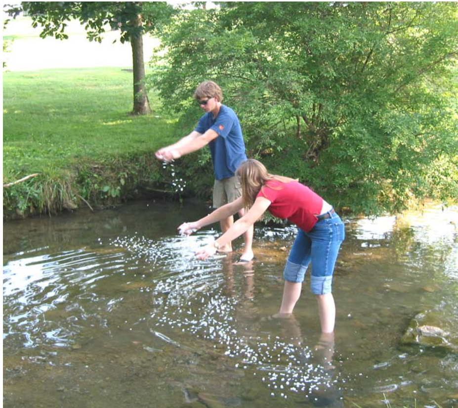
Figure 23. A photo showing starch packing material being applied to the water surface in low-flow conditions. Starch packing material served as the tracer particles for the LSPIV prototype.
