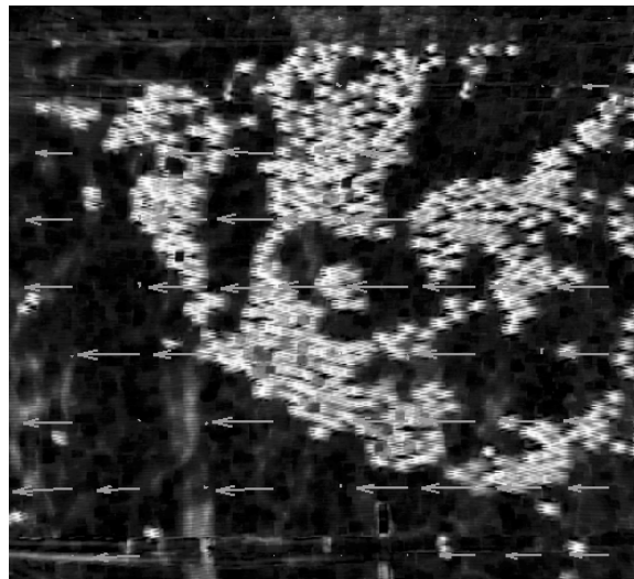
Figure 14. Surface velocity field produced by one image pair from laboratory experiments. The grid spacing interrogation window sizes were chosen to provide adequate resolution without being too computationally intensive.
