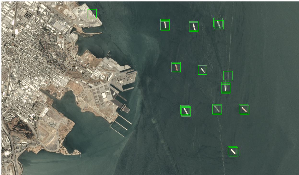
Figure 5.4: The output of the ship detection algorithm on the image Sfbay_3. The green boxes represent image chips classified as a ship. There are a few false positives, but no missed ships.
