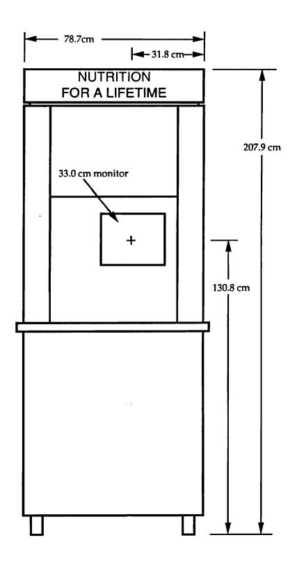
Figure 1. Front view of the Nutrition for a Lifetime kiosk.
