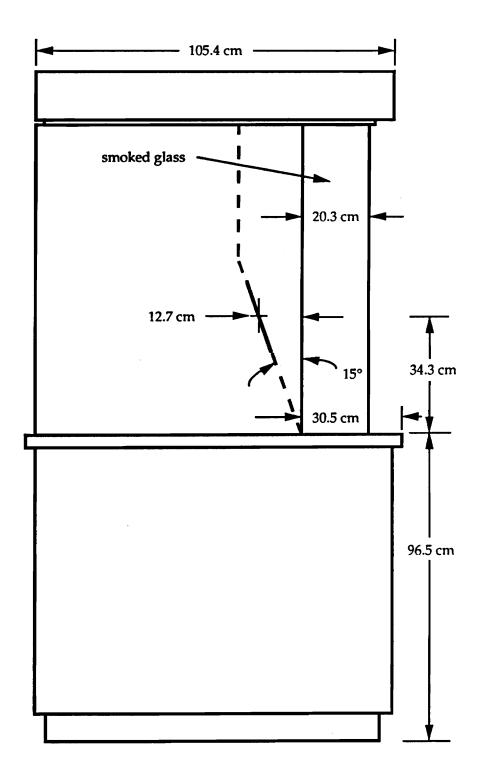
Figure 2. Side view of the Nutrition for a Lifetime kiosk.
