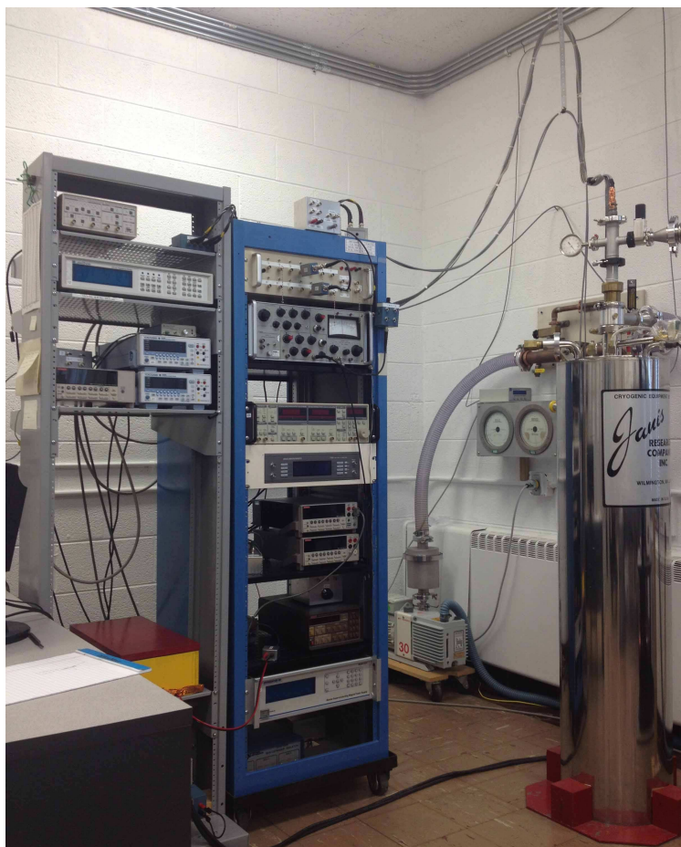
Figure 2.6: Equipments on the left shelf are LakeShore 370 AC resistance bridge, Princeton Applied Research P124A analog lock-in amplifier, SR 830 digital lock-in amplifier, EG&G 7265 digital lock-in amplifier, Keithley 2400 source meter, Keithley 2000 multimeter, Cryomagnetics CS-4 superconducting magnet power supply. On the right is the cryostat system.
