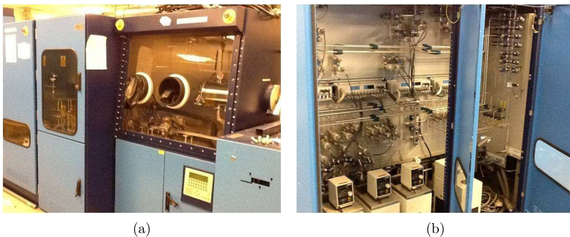
Figure 2.1: Aixtron 200/4 RF-S MOCVD system. (a) Reactor and glove box. (b) Material sources.
