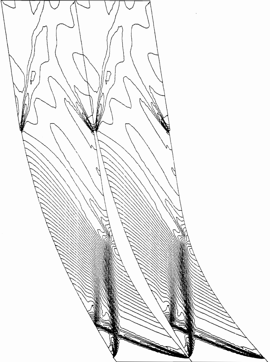
Figure 28. Contour Plot of Static Pressure at Design Incidence, Calculated
