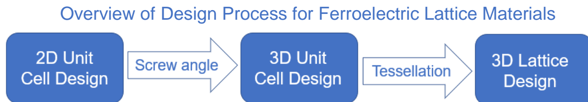
Figure 7. High-level overview of the ferroelectric lattice material design process.
