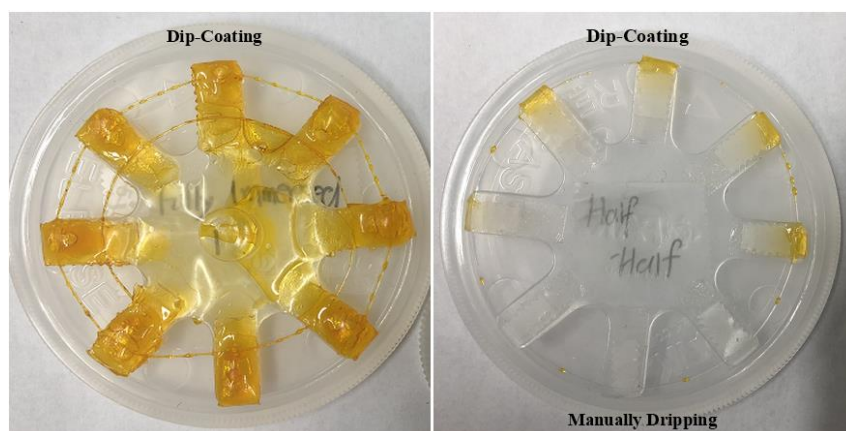
Figure 38. Dip-coating with PEGDA drawback. LEFT: Dip-coating creates a thick layer of PEGDA all over the plastic frame. RIGHT: Compare dip coating (top half) with manually dripping (bottom half), the bottom half is neater than the top half.
