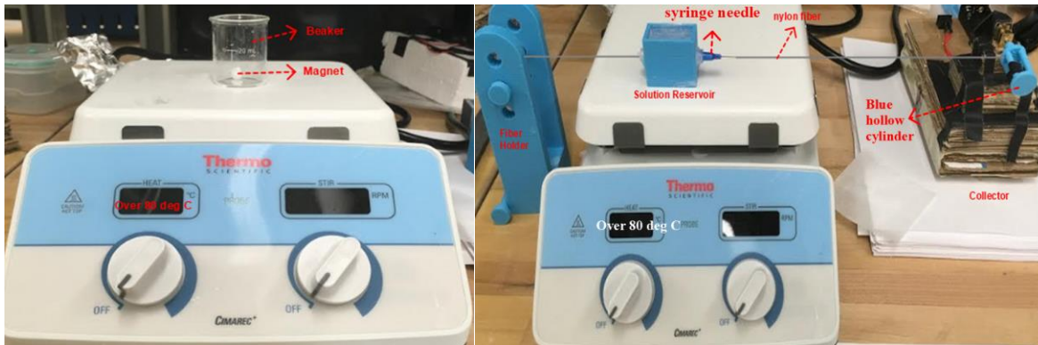
Figure 16. Fluid Coating Setup. Left: Preparing the PMMA solution. Right: Fiber drawing to form Spindle-Knot. The motor drives the blue hollow cylinder clockwise to draw the fiber out of the solution reservoir. The collecting speed can be controlled by replacing different hollow cylinder size. The drawing speed can control the fluid coating layer thickness.
