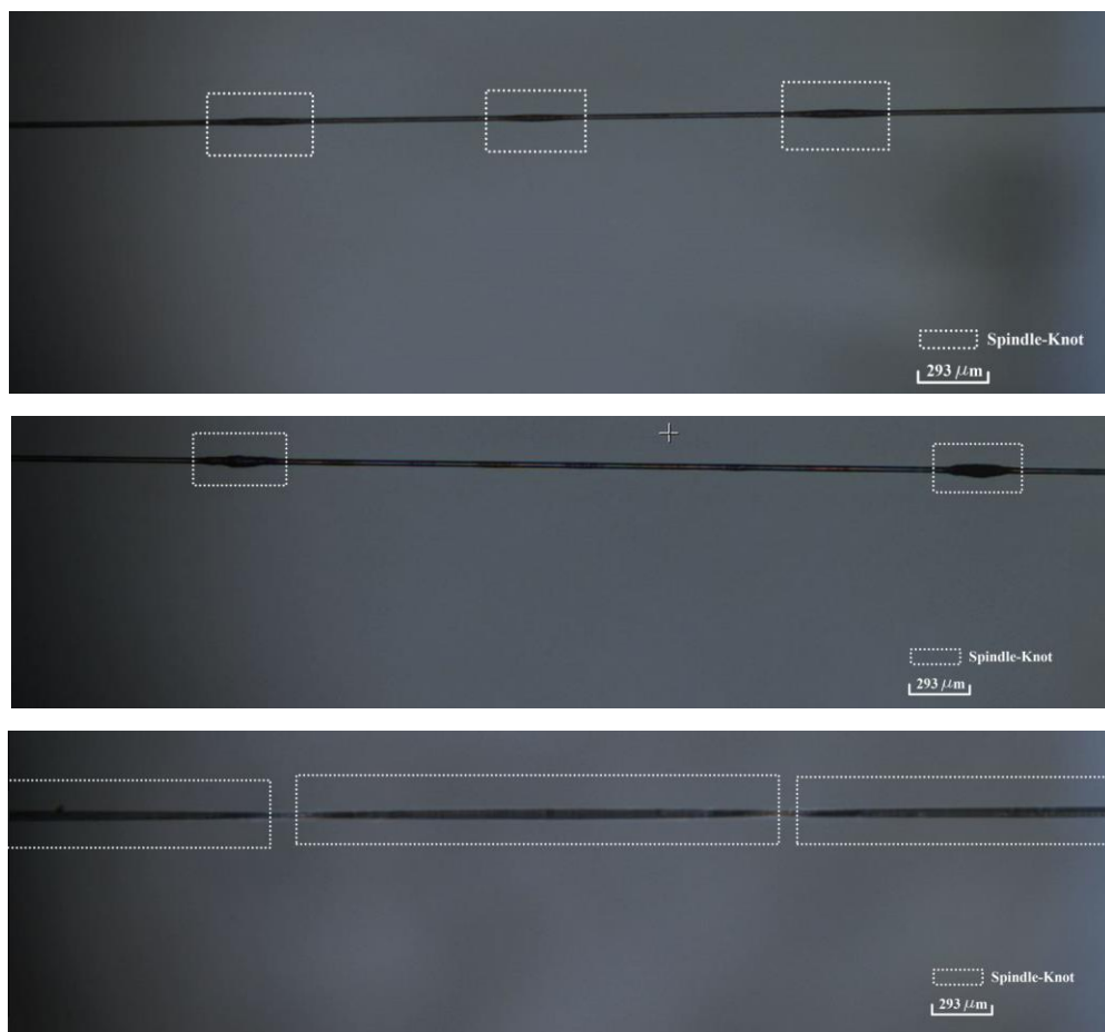
Figure 17. Nylon fiber fluid coating. Less than 15% of the trials form the spindle-knot, and they all form different spindle knot sizes and thicknesses.
