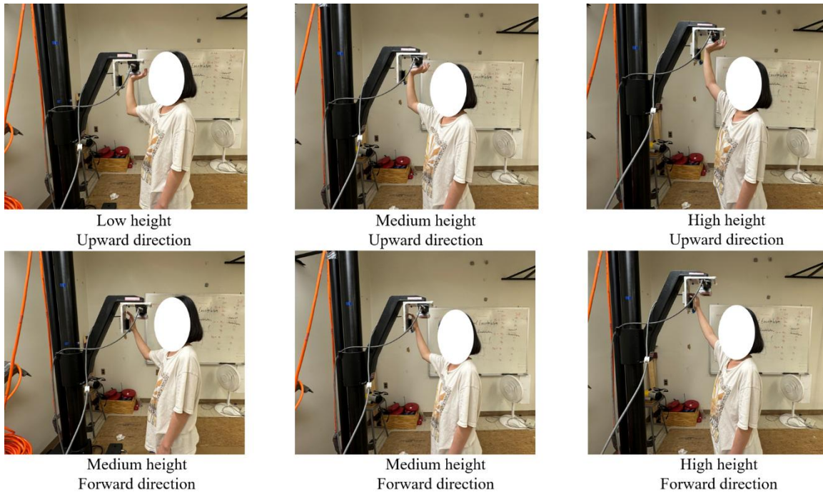
Figure 1. Illustration of six simulated task conditions (three work heights and two push directions).
