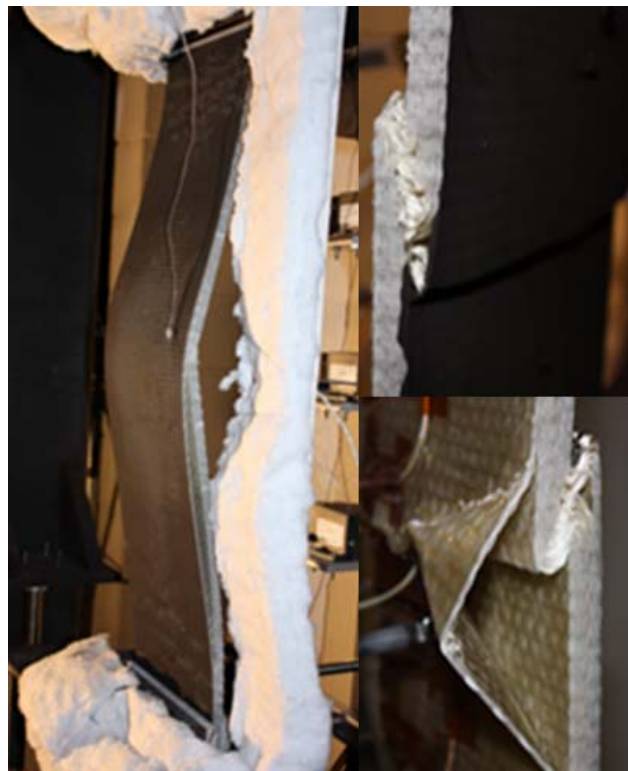
Figure 1.4: Compressive failure modes of PMCs exposed to fire (used with permission of Patrick Summers [134])
