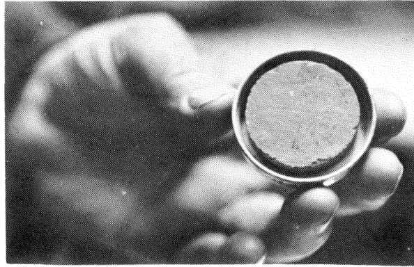
Figure 8—When it dried, this plastic clay shrank away from the edge of the container. Clays of this kind will cause damage to foundations, roads, streets, parking lots and swimming pools by shrinking when dry and swelling when wet. Some critically shrinking clays will shrink 6-7% of their volume from wet to dry and swell back when wet.
