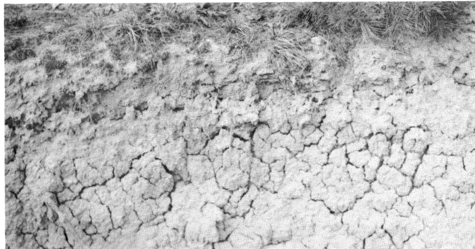
Figure 10—This is Helena fine sandy loam, which has a sandy surface and extremely plastic, sticky, clayey subsoil.
