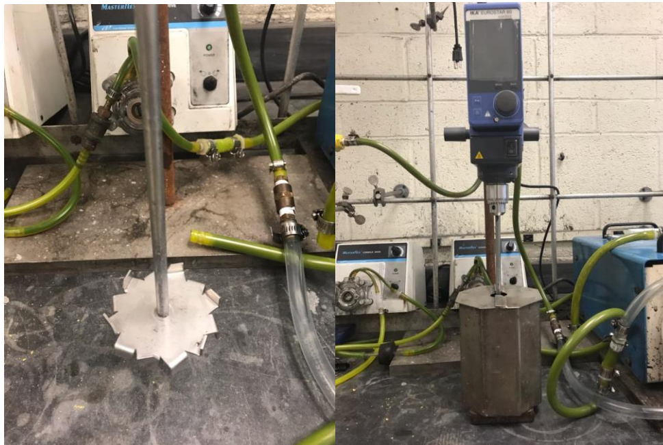
Figure 4-24: (Left) blunging impeller, (Right) blunging mixing vessel
