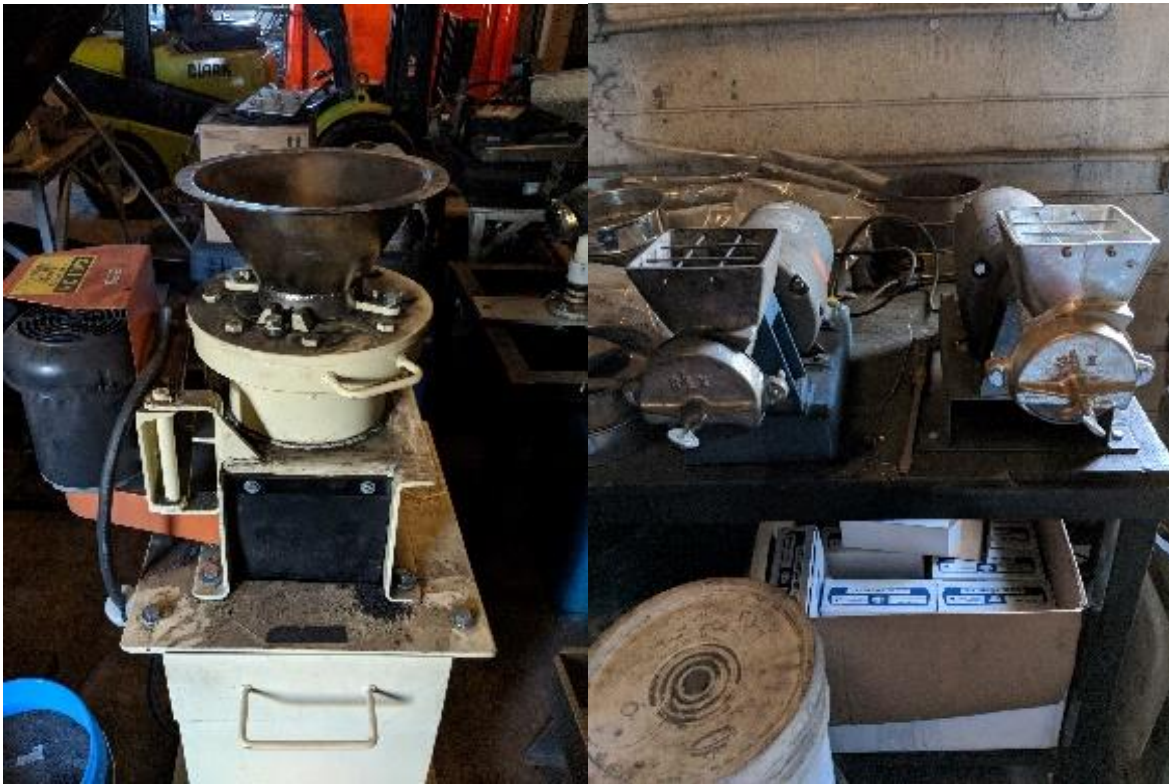
Figure 4-2: (Left) laboratory cone crusher, (Right) laboratory coffee grinder
