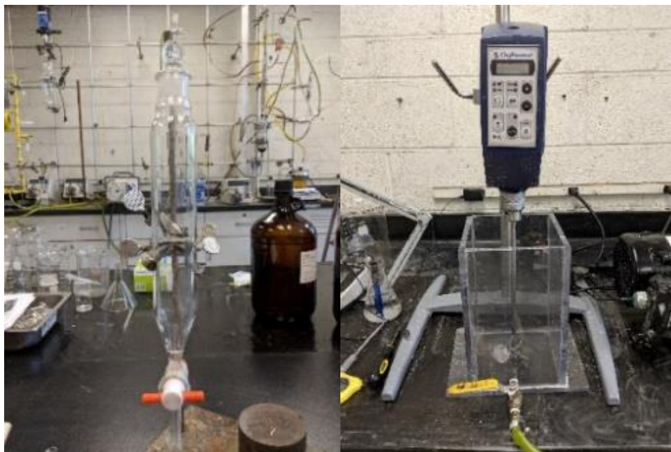
Figure 5-2: (Left) separatory funnel for hand shaking tests (Right) Plexiglas tank for conditioning and emulsion formation
