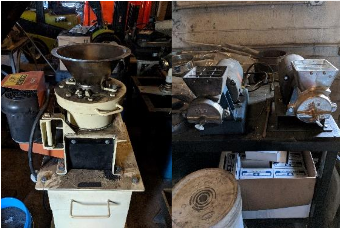
Figure 3-2: (Left) laboratory cone crusher, (Right) laboratory coffee grinder
