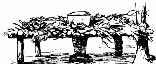
THIS HOPPER FEEDER FOR SMALL GAME IS DEER- PROOFED BY ERECTING AROUND IT A 12'-14' SQUARE ROOF. THE ROOF IS ONLY 2 FT. ABOVE THE GROUND TOO LOW TO ADMIT DEER. 4 STURDY POLES SET ON POSTS SUPPORT THE CROSS POLES & COVERING.
