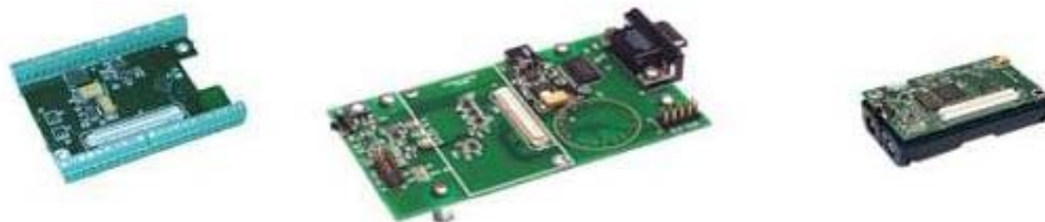
Figure 4.4: Data logger (MDA300) (left), Base station (MIB510) (middle), and Transceiver (MPR410CB) (right)
