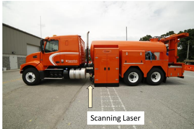
Figure 17: Sideway-Force Coefficient Routine Investigation Machine (SCRIM) equipped with a scanning laser (sampling frequency 64 kHz) used to measure the pavement profile.
