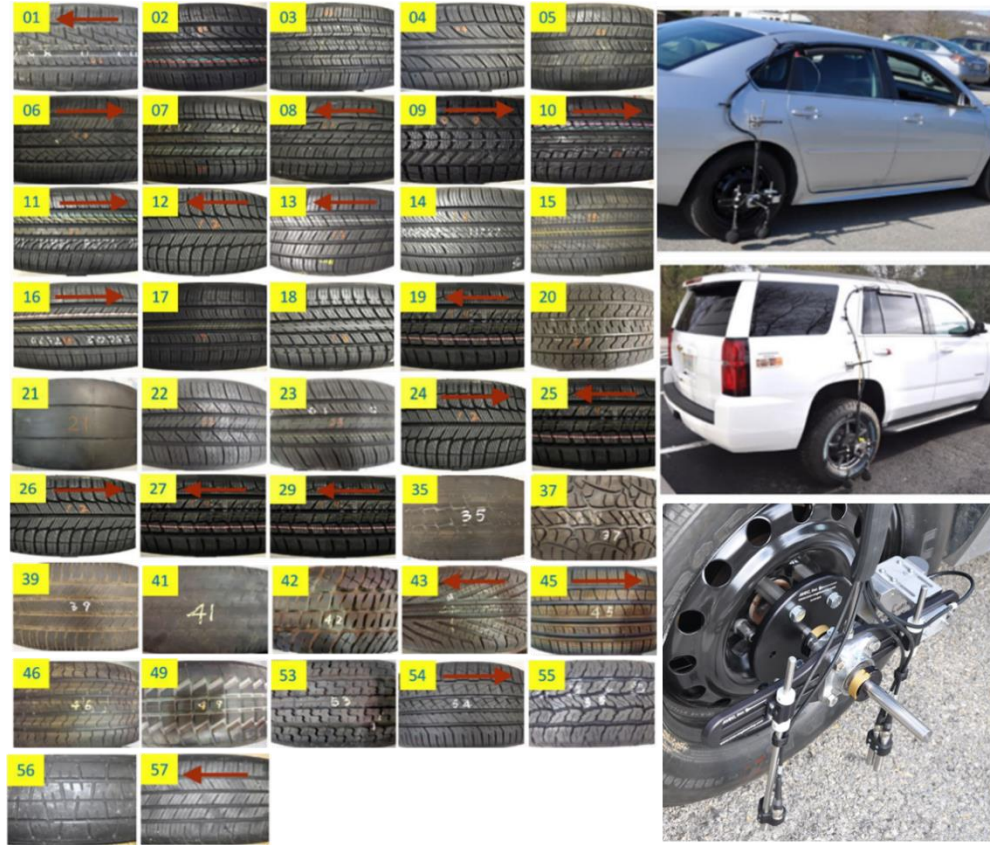
Figure 20: 42 tires tested, 2 vehicles used, and OBSI system with optical sensor implemented for the U.S. Route 460 test.
