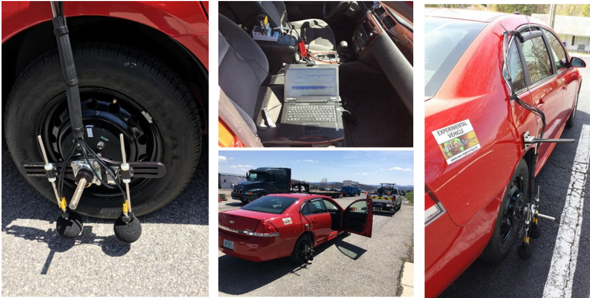
Figure 78: Pictures of tire noise test on the SMART road
