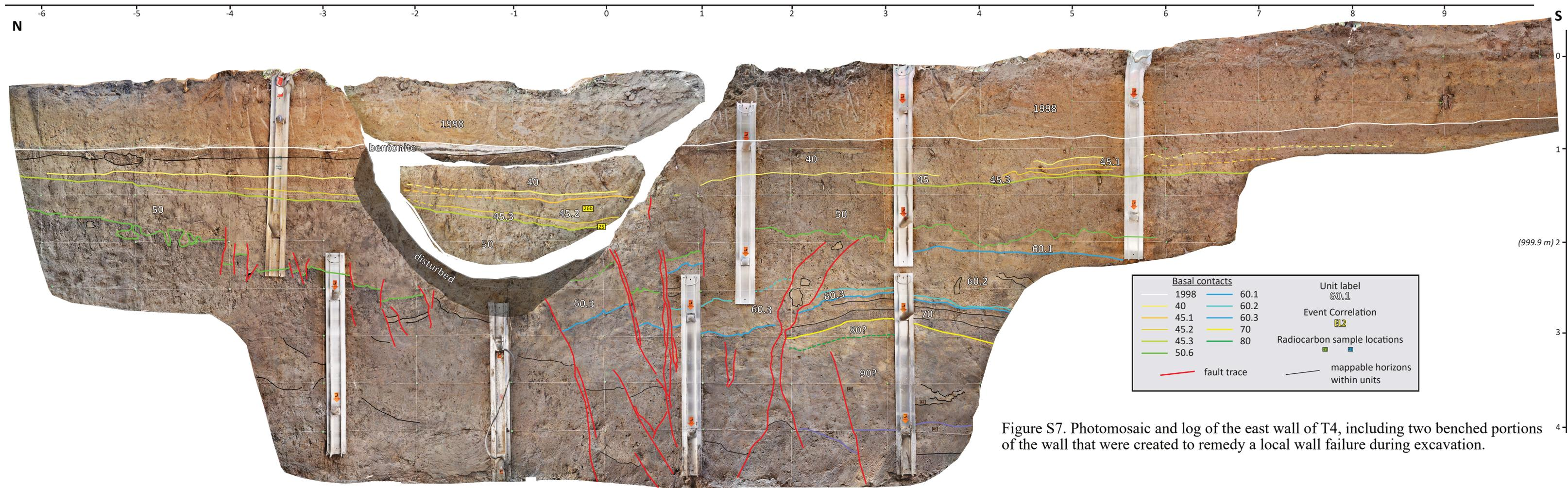
Figure S7. Photomosaic and log of the east wall of T4, including two benched portions of the wall that were created to remedy a local wall failure during excavation.
