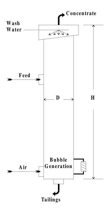
Figure 1.1: Flotation Column Layout
