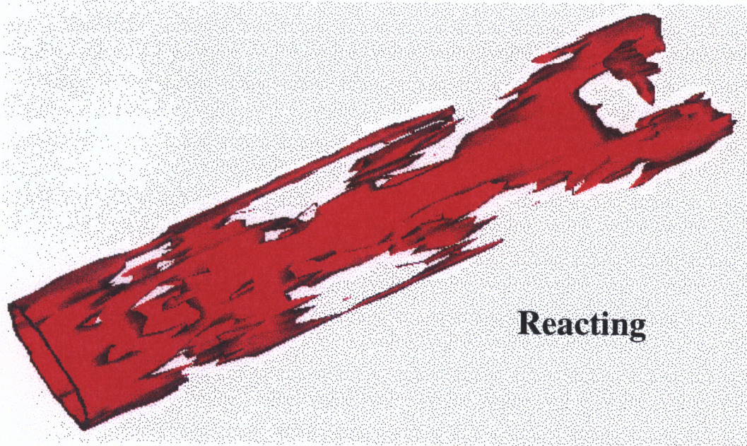
Figure 5.10. Iso-surfaces of both the reacting and nonreacting elliptical jets: iso-level = 29000 1/sec (apx. 1/2 maximum vorticity)
