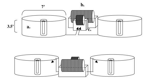
**Figure 4.2.** Fingerling production system: **a-** rearing tank (1,000 gal ea), **b-** RBC biofilter, **c-** rotating screen filter.
