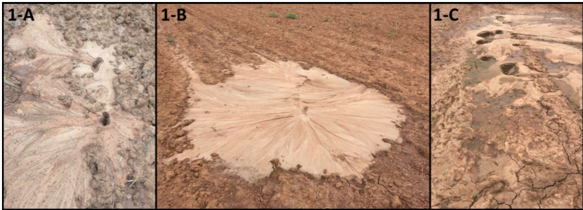
Figure 3.2. Photos of liquefaction manifestations at Test Site 1 (Photos courtesy of Dan Ripley).
