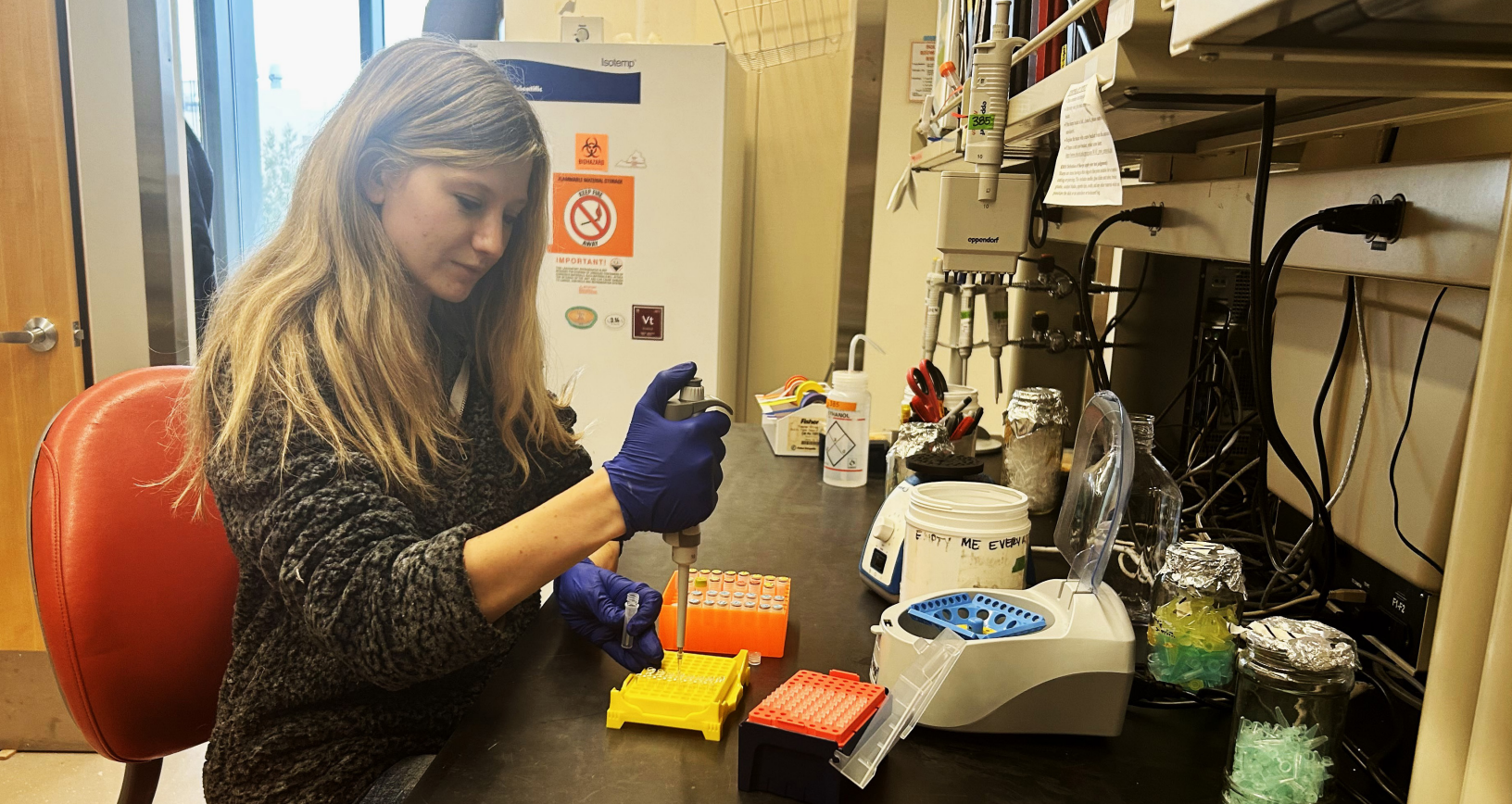
Amanda Darling prepares a plate for ddPCR which is a method used to detect pathogens in water and wastewater samples. Photo provided by Amanda Darling.
