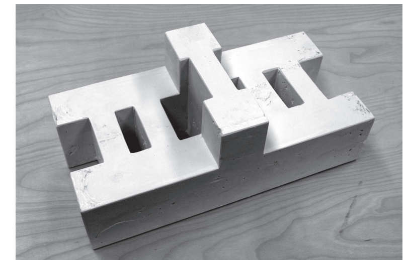
A T-shaped brick was developed to increase the connection between masonry courses and to express a tectonic nature of the walls; the woven brick helps the wall act more like vault
