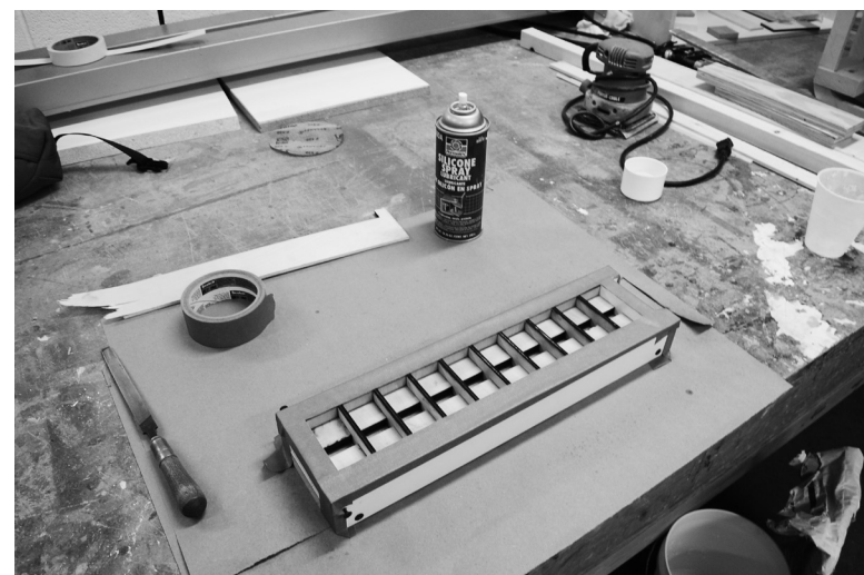
Reusable wood formwork allows casting 10 units at a time at 1:8 scale
