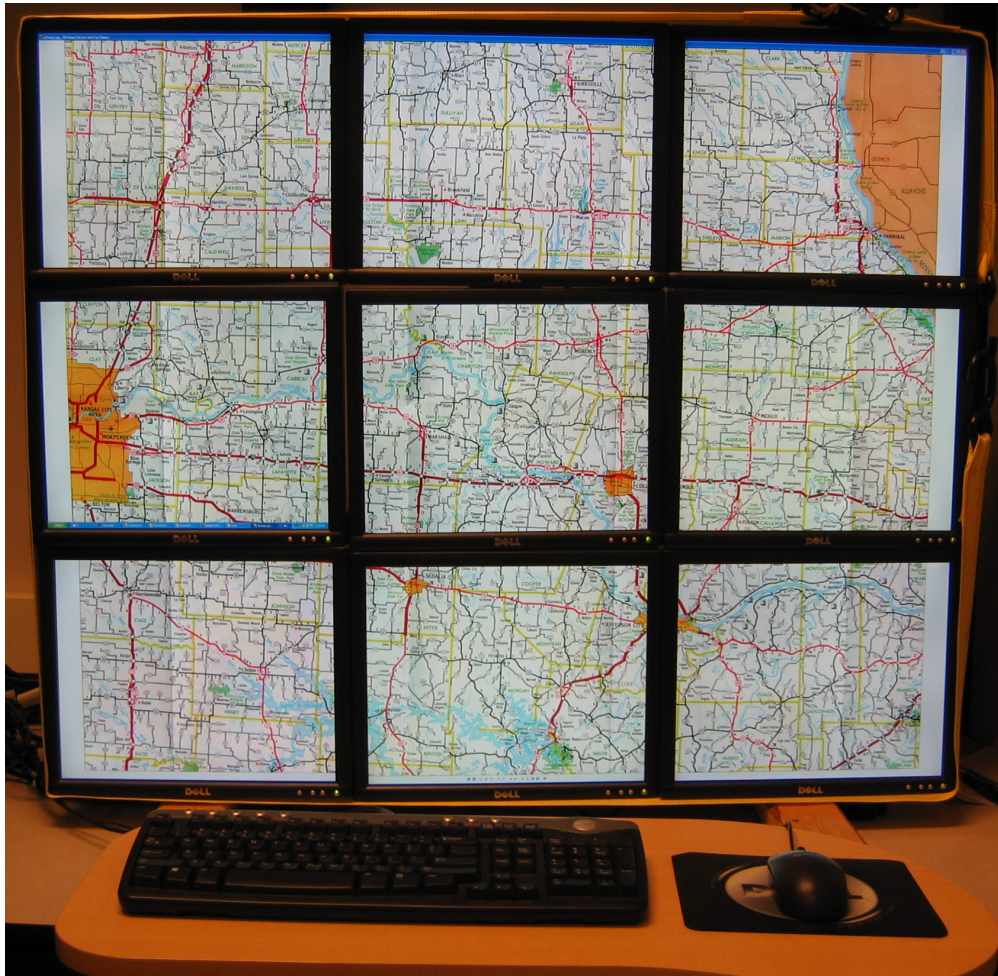
Figure 3.2. Multiple monitor display constructed of nine 17" flat screen LCDs (3840 x 3072 pixels). Note the presence of bezels in the interior of a multi-display system because of current display technology for LCD panels.
