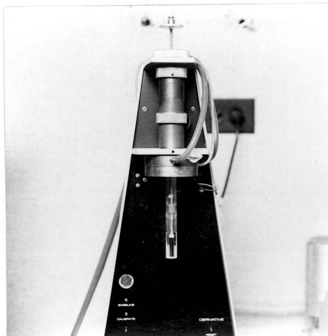
Figure 3. Apparatus for thermal expansion analysis.
